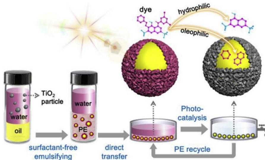
Figure 18. Schematic representation of photocatalytic dye degradation in O/W Pickering emulsion stabilized by commercial TiO 2 NPs. The dye molecules attached on the surface of TiO 2 and tuned its wettability to be an emulsifier. (Ref 148 with permission from Elsevier)
