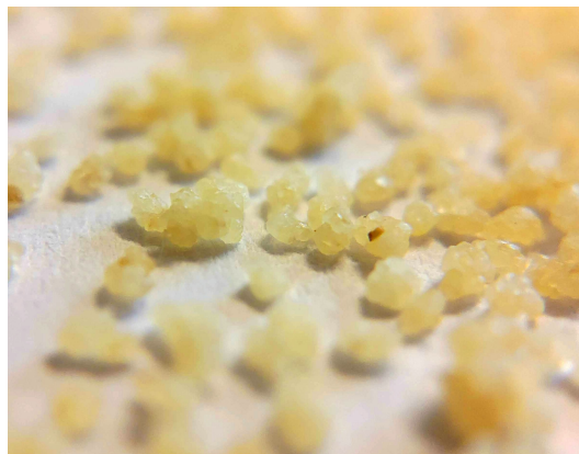
FIGURE 2.1: Particles of the fine couscous chosen as the reference water sensitive granular material. The picture highlights the complicated particle shape, formed by several semolina grains gelatinised together.
