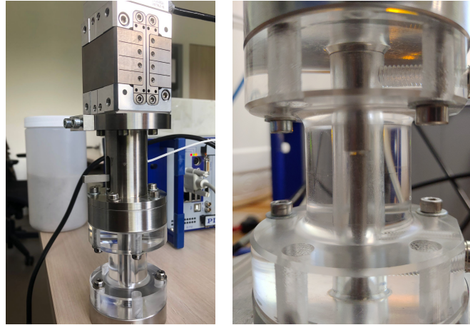
FIGURE B.2: Pictures of the compression setup used to test individual couscous particles. On the left, the whole mounted apparatus. On the right, a detail showing the particle positioned between the two pistons.
