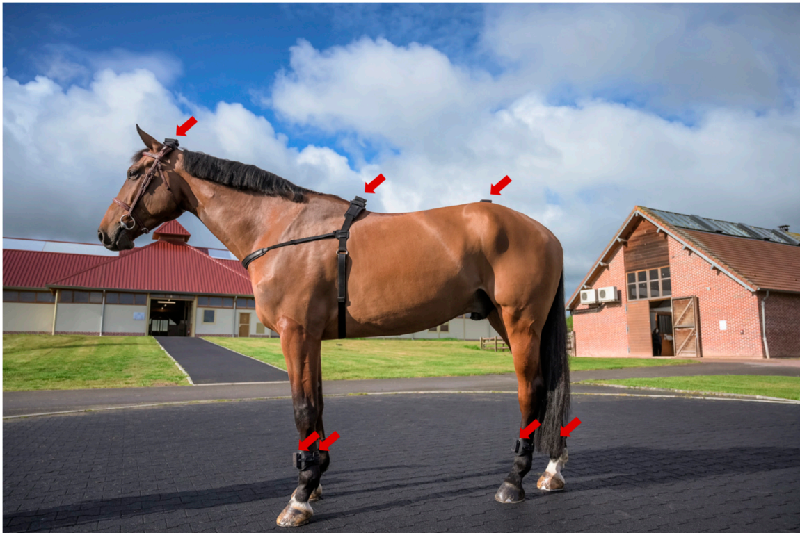
Figure 1. Horse equipped with EQUISYM ® system, composed by sensors placed on the head, the withers, the pelvis and the four cannon bones (shown by the red arrows).
