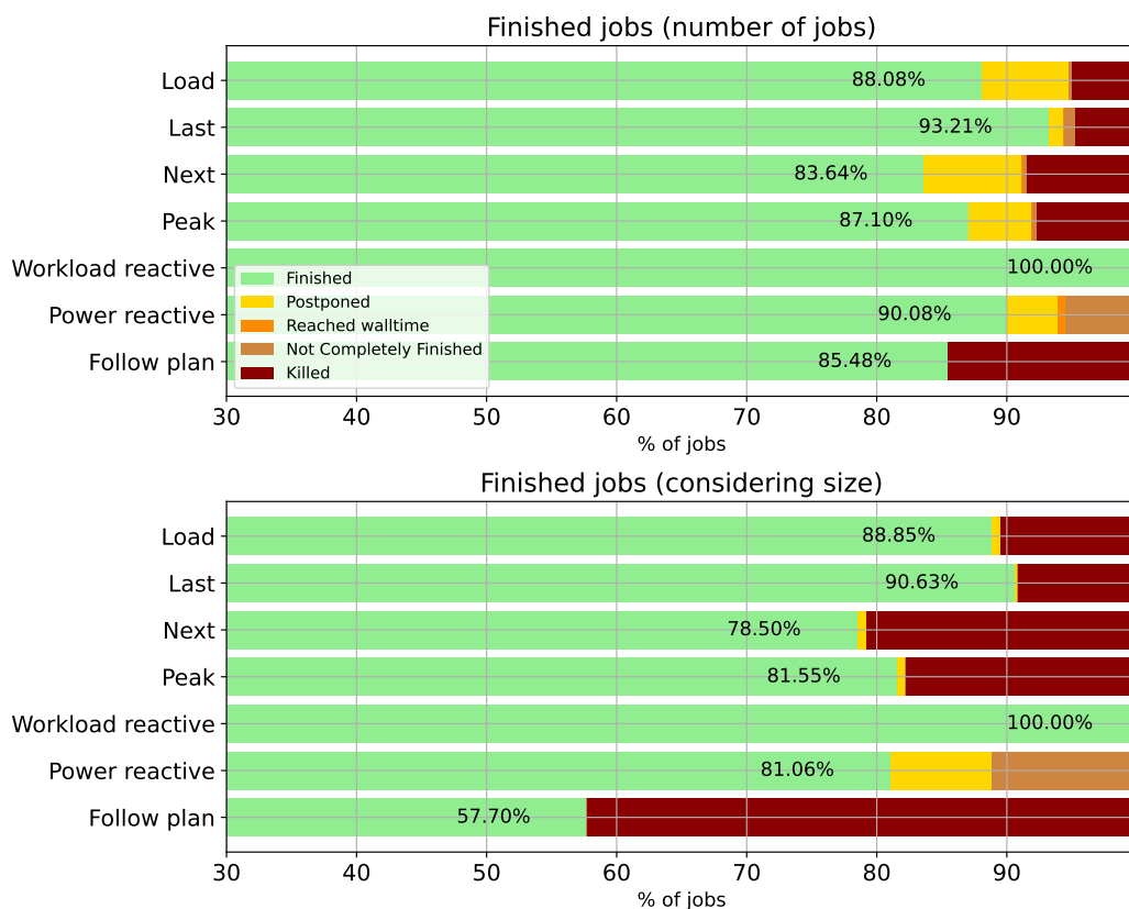
Figure 4.14: Jobs state at scenario Critical 2. The first graph (above) considers only the number of jobs, ignoring their size. In the second graph (below), the jobs' size is considered.
