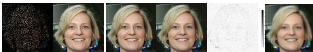
Figure 5.4: Image inpainting, from left to right: measurement, true image, MMSE estimate \hat{\mathbf{x}}_{\text{MMSE}} , MMSE estimate \hat{\mathbf{z}}_{\text{MMSE}} , pixel-wise 90% credibility intervals, averaged samples generated by MCG [159]
