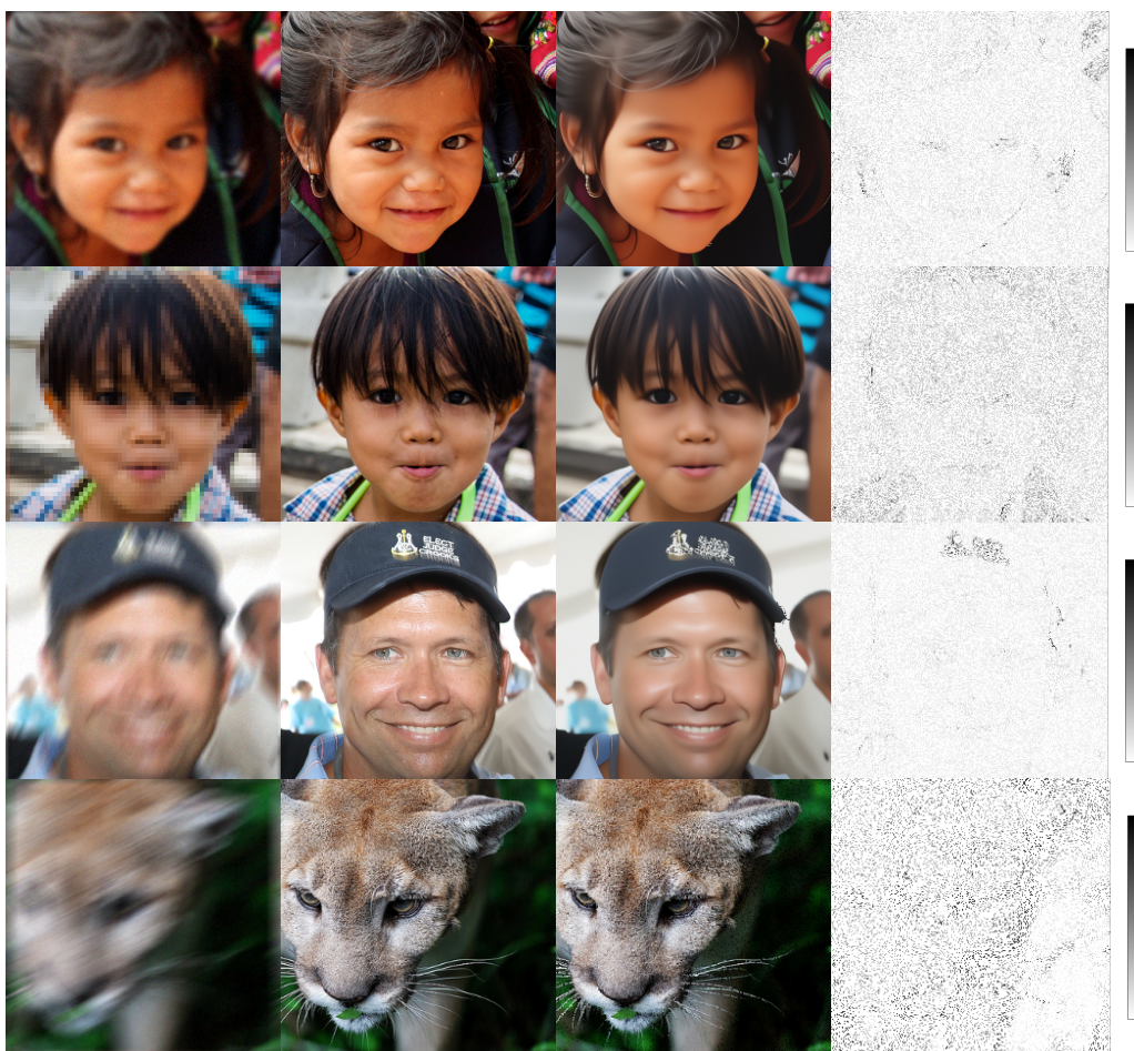
Figure 5.3: From left to right: measurement, true image, MMSE estimate, pixel-wise 90% credibility intervals. From top to bottom: Gaussian blur, superresolution and two motion blurs. The first three and the last images are from the FFHQ and Imagenet data sets, respectively.
