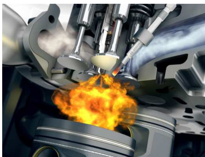
Figure 1.2. Schematic of a Diesel engine performing combustion
