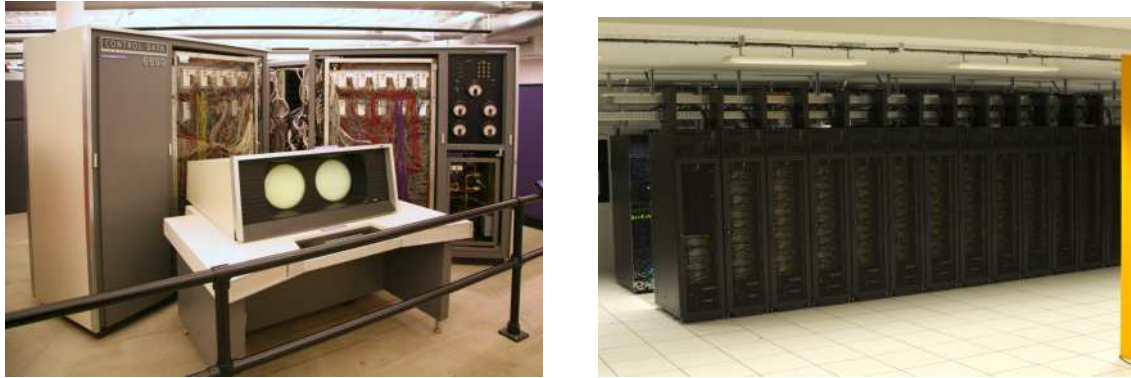
Figure 1.3. On the left side the supercomputer CDC 6600 with its console, launched in 1964, and on the right side the supercomputer Occigen installed by GENCI at CINES, in Montpellier; with which the databases presented in this thesis were obtained.
