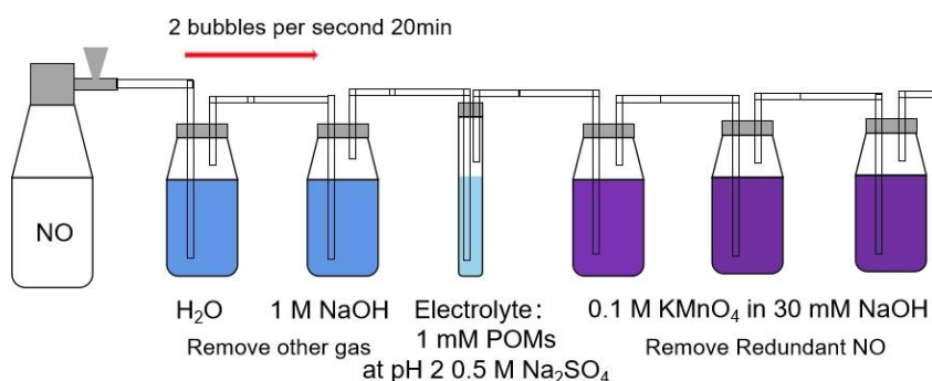
Figure A.1 Experimental design for safely bubbling of NO into a POM containing electrode.
