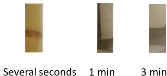
Figure 3.4.3 Picture of \text{Ag}@[ \text{PW}_{12}\text{O}_{40} ]^{3-} NPs obtained with a different addition time of the \text{Ag}^+ solution into the photoreduced POM solution.
