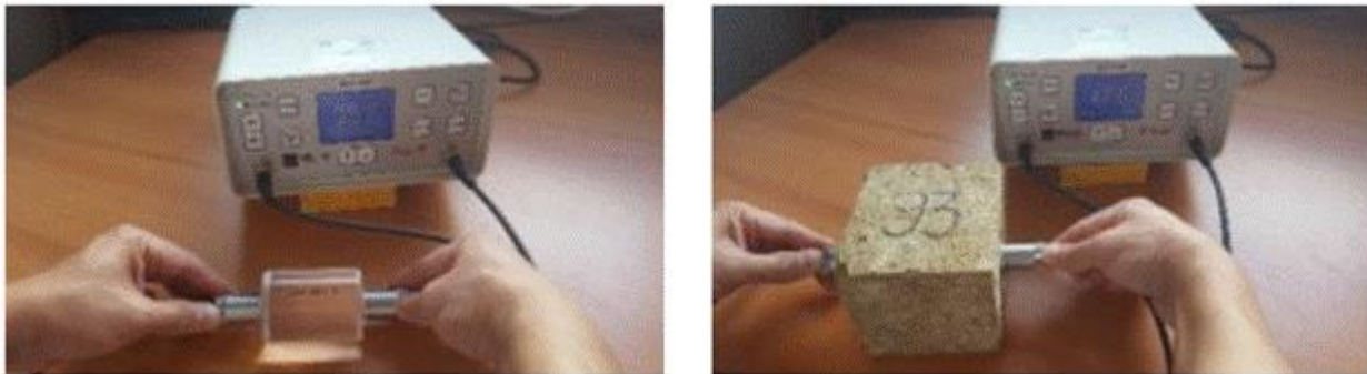
Figure 2.15: Ultrasonic pulse velocity test (calibration and measurement) (Ngo, 2017)
