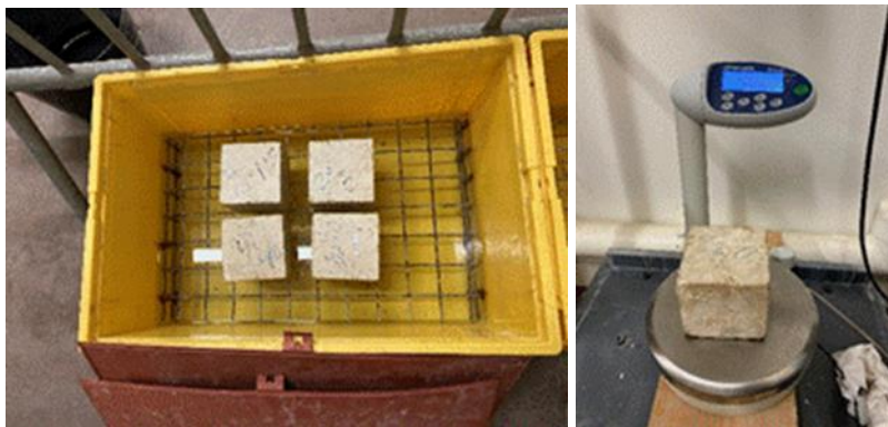
Figure 2.17: Capillary rise test procedure
