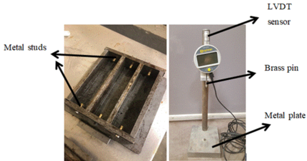
Figure 2.16: Molds with metal studs and shrinkage tests device
