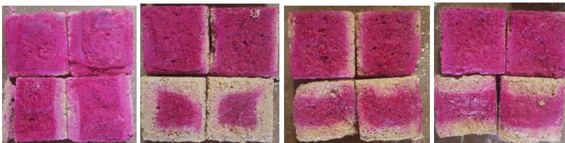
Figure 2.28: Carbonation at 120 days. From right to left: NS30/70, RS20/80, RS30/70 and RS40/60 where the upper and lower raw correspond to the specimens at wet and drying curing conditions, respectively.
