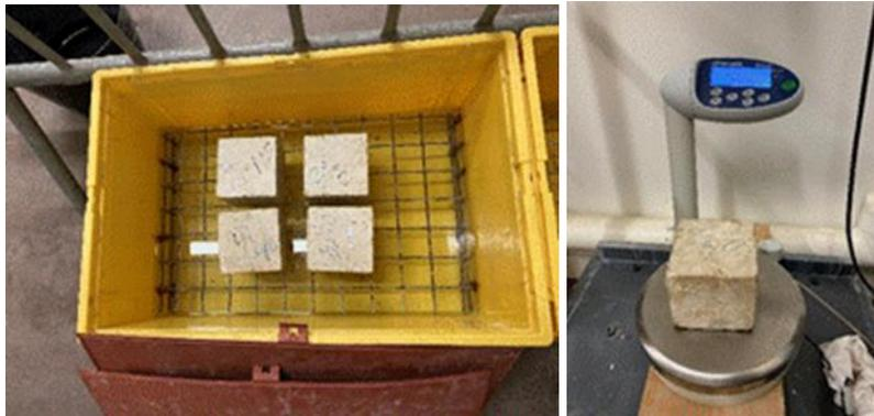
Figure 2.17: Capillary rise test procedure
