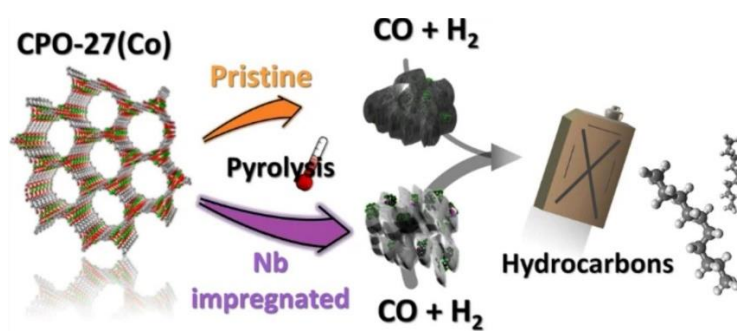
Figure I-28. Post-synthesis impregnation with niobium(V) oxalate precursor into CPO-27(Co) and its application in Fischer–Tropsch synthesis catalysis. [88]
