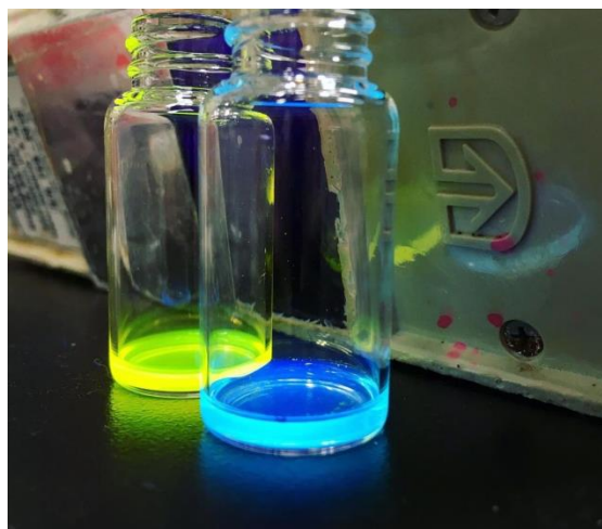
Figure 7: Two modified BODIPY® fluorophores in dichloromethane upon UV excitation.
