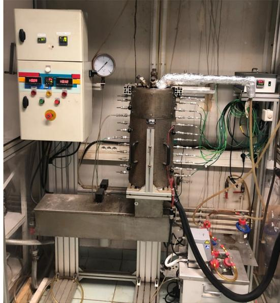
Figure 2.7: Fixed-bed reactor used in pyrogasification experiments
