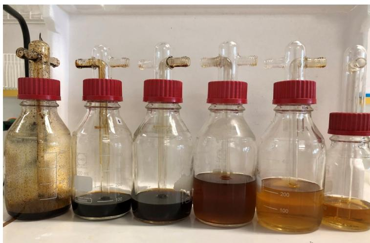
**Figure 2.9:** Collected condensates during pyrolysis stage
