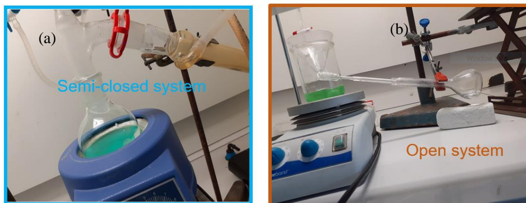
Figure 5. 8. \text{HNO}_3 recovery after Ni/NiO leaching from the electrode electrolyte assembly of SOFCs (a) semi-closed system (b) open system.
