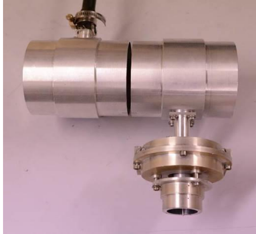
Figure 44. Thruster connected to custom in-vacuum microwave transmission line used in this study. A corresponding schematic view is in figure 41, right.
