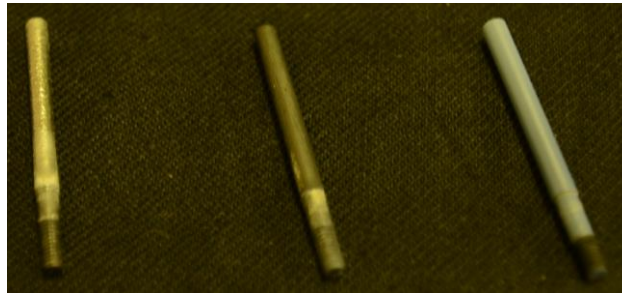
Figure 86. Some of the tested inner conductors. From left to right: boron nitride spray (partly peeled after operation), graphite, pyrolytic boron nitride deposited on graphite. Being translucent but diffusing blue light, this material appears slightly blue on graphite.
