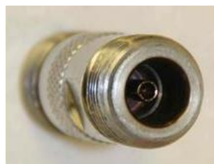
Figure 42. N-connector that is screwed to the thruster, after operation.
