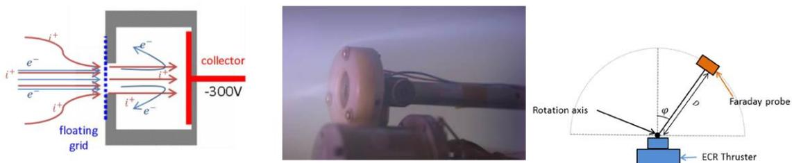
**Figure 36.** Measurements with a gridded Faraday probe. Reproduced from [24].
