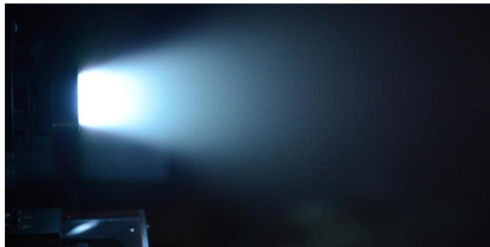
Figure 74. ECRT firing at JLU, mounted on the thrust balance.
