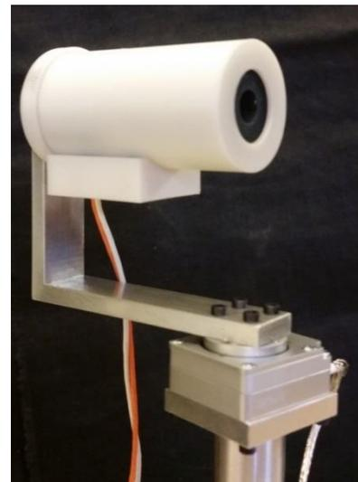
Figure 70. Directional probe with two degrees of rotation.
