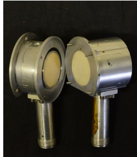
Figure 112. Picture of the microwave test setup. On the left is the coaxial-to-waveguide transition used in the thruster. On the right are test parts.
