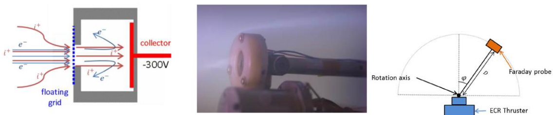
Figure 36. Measurements with a gridded Faraday probe. Reproduced from [24].
