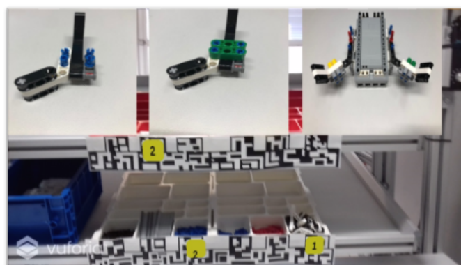
Fig. 4.3 Example of the images that appear on the HMD to the operator, when he/she looks at the bins [124].
