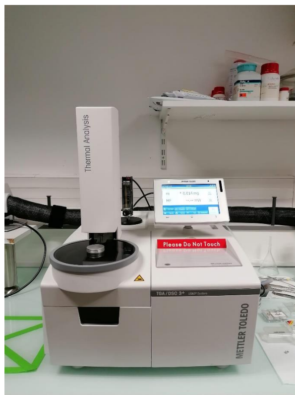
Figure 3.2. MATTLER TOLEDO TGA/DSC 3+ instrument, installed at the ISTerre (UGA).
