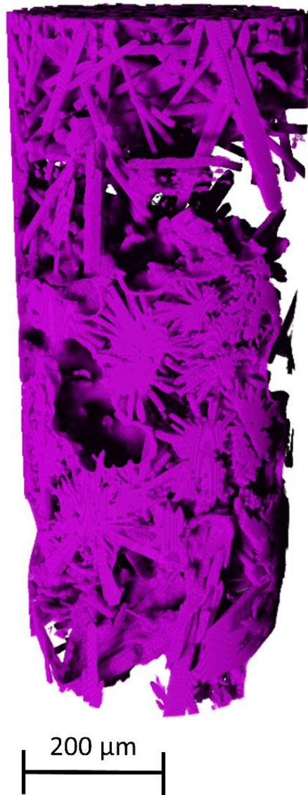
Figure 4.43. 3D reconstruction of the sample after 4 hours of hydration. The volumes shows two distinct regions. The top part of the sample was not hydrated and shows a concentration of quartz wool fibres and few hemihydrate crystals. The middle and bottom part of the volume shows the region that was hydrated which at this point of the hydration is characterized by the presence of agglomerates of gypsum needles.
