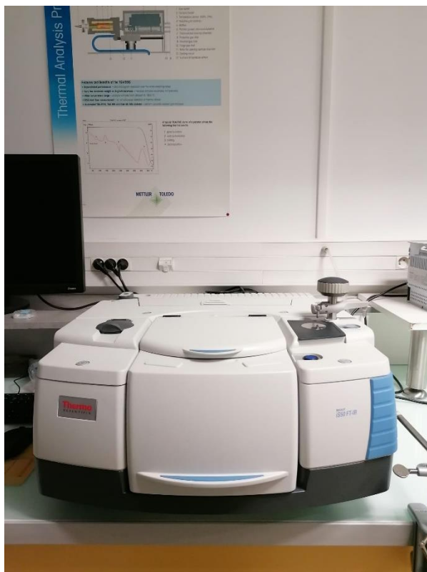
Figure 3.7. Nicolet iS50 FTIR spectrometer, installed at the ISTerre (UGA).
