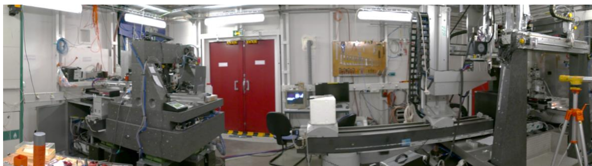
Figure 3.12. Panoramic of EH3 at the ID11 beamline. The beam enters the hutch from the right. The first end-station is the 3DXRD microscope. The second one on the left is the nanoscope.
