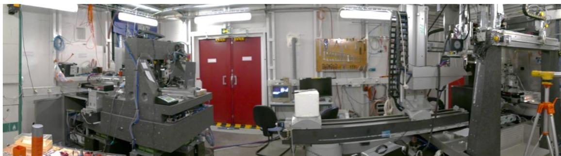
**Figure 3.12.** Panoramic of EH3 at the ID11 beamline. The beam enters the hutch from the right. The first end-station is the 3DXRD microscope. The second one on the left is the nanoscope.
