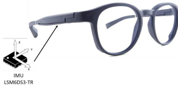
**Figure 1.** Placement of the IMU in the branch of the smart eyeglasses
