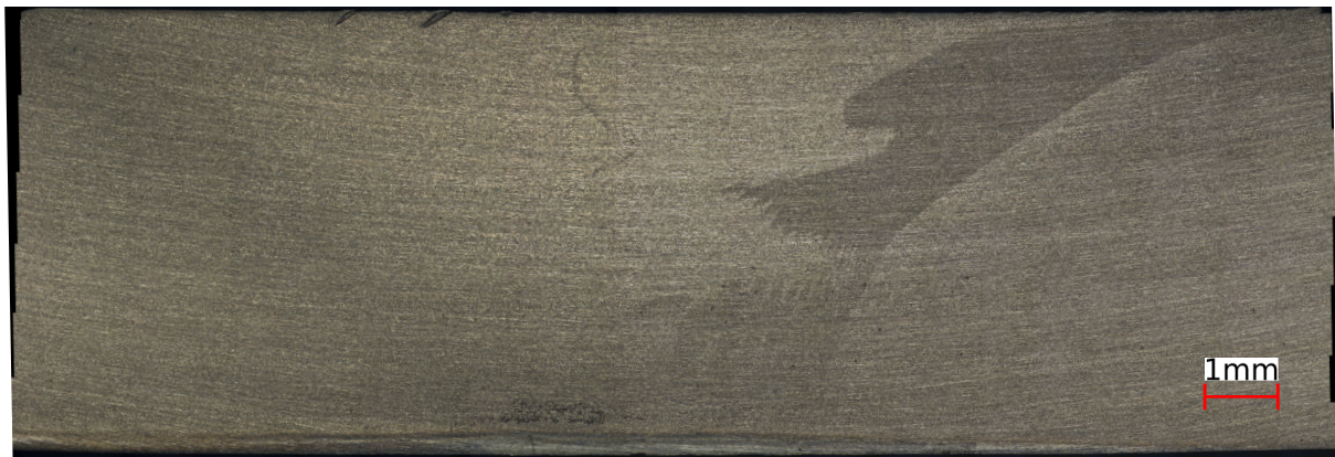
Figure IV.1: Example of a similar Al/Al AA7075 joint under optical microscopy, after etching with Weck's reagent.
