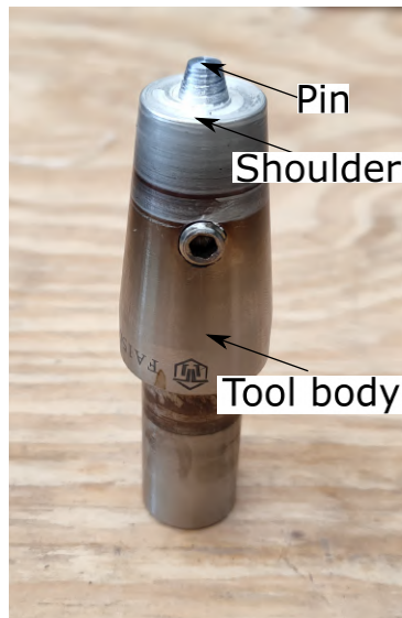
Figure I.1: A typical FSW tool made of tooling steel. The pin stirs the material as the shoulder generates the majority of the heat input during welding.
