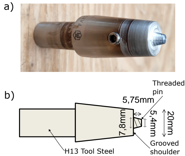
Figure II.8: (a) Picture of the FSW Al/Al tool used (b) Schematic of the steel FSW tool used in the manufacturing of aluminium similar and dissimilar joints.
