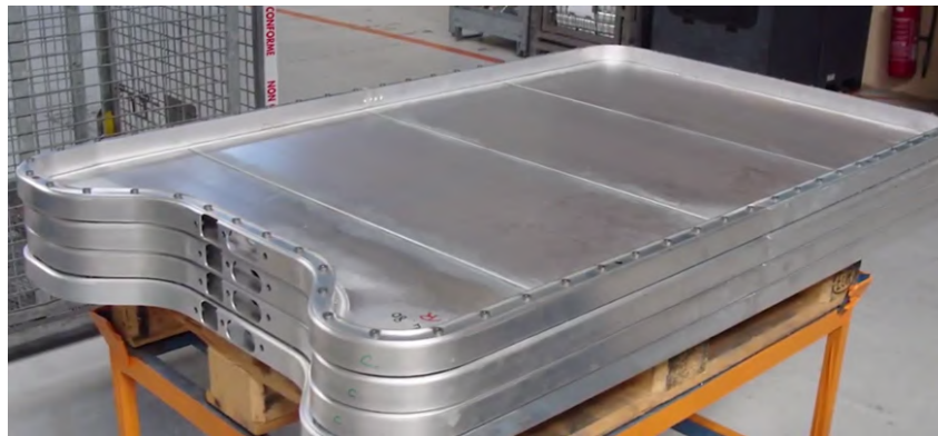
Figure I.15: Battery tray of the Renault Zoé. The tray is assembled via FSW from extruded aluminium. FSW adds mechanical strength and the guarantee of a sealed joint. [41]
