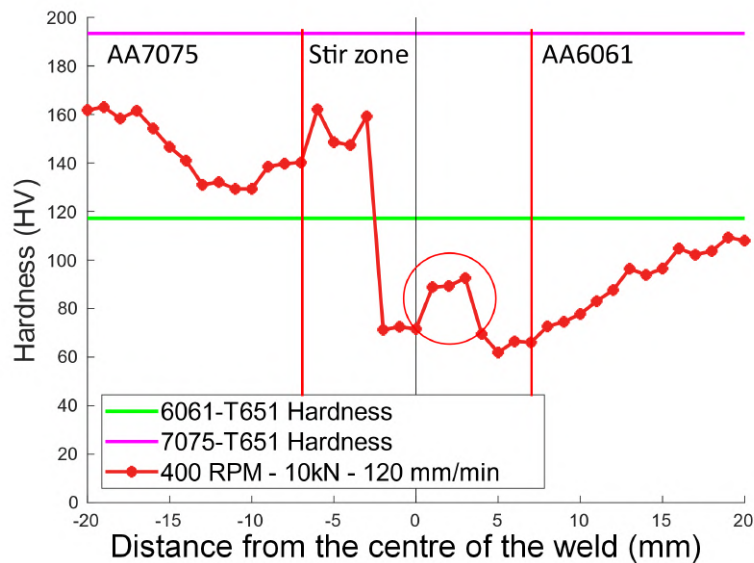
Figure IV.44: Hardness profile taken at the centre line of the studied AA6061-AA7075 FSW joint. The HR-DIC sample has been extracted in the red-circle zone.
