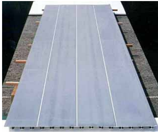
Figure I.12: Friction stir welded floor panels produced by Sumitomo Light Metal for the 700 Series Shinkansen (see Figure I.13) [39].
