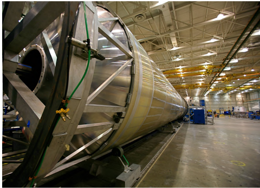
Figure I.8: A Space X Falcon 9 booster tank assembled in FSW [34].
