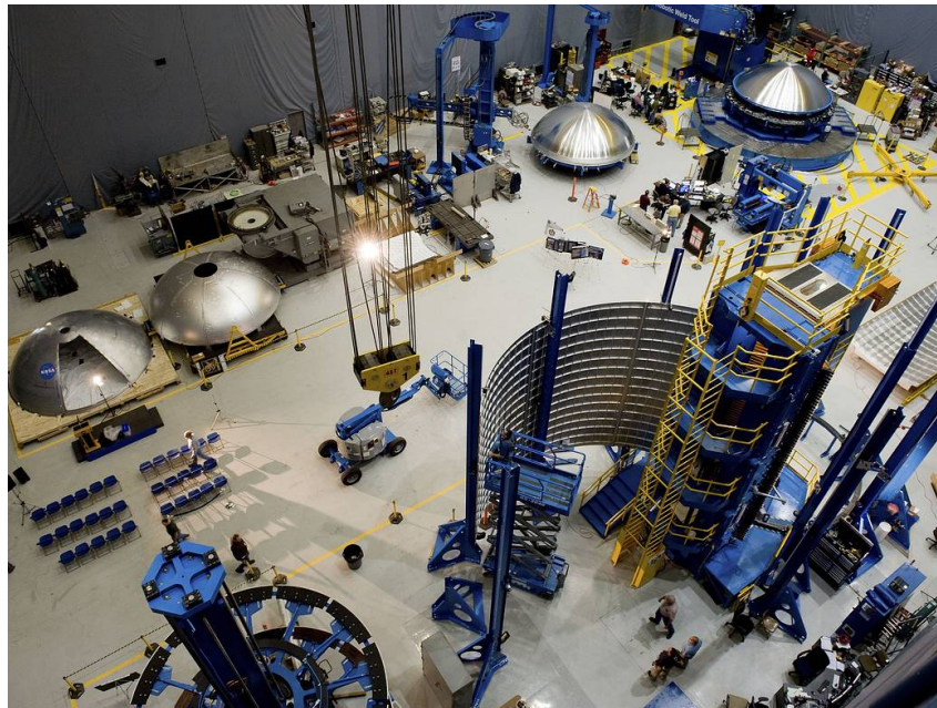
Figure I.7: Four aluminum domes, each created using FSW, are seen in this overhead view of the Marshall Space Flight Center Advanced Welding and Manufacturing Facility [33].
