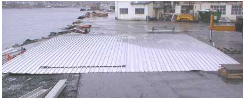
Figure I.10: Prefabricated FSW panel for a catamaran sidewall. Straight panel for ship transportation at Marine Aluminium in Haugesund, Norway [37].
