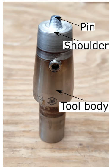
Figure I.1: A typical FSW tool made of tooling steel. The pin stirs the material as the shoulder generates the majority of the heat input during welding.
