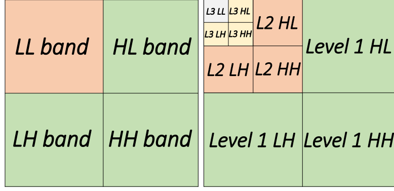
Figure 3.3: Wavelet coefficients generated by 2-D DWT. Left: 1-level decomposition. Right: 3-level decomposition.
