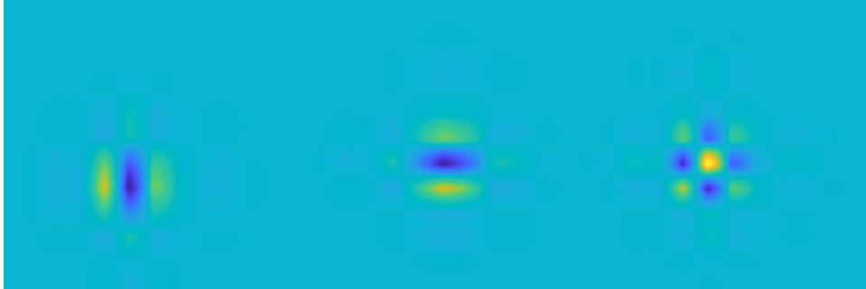
Figure 4.2: db4 wavelets (LH, HL, HH) associated with the 2-D DWT in the space domain. Level of decomposition is 5.
