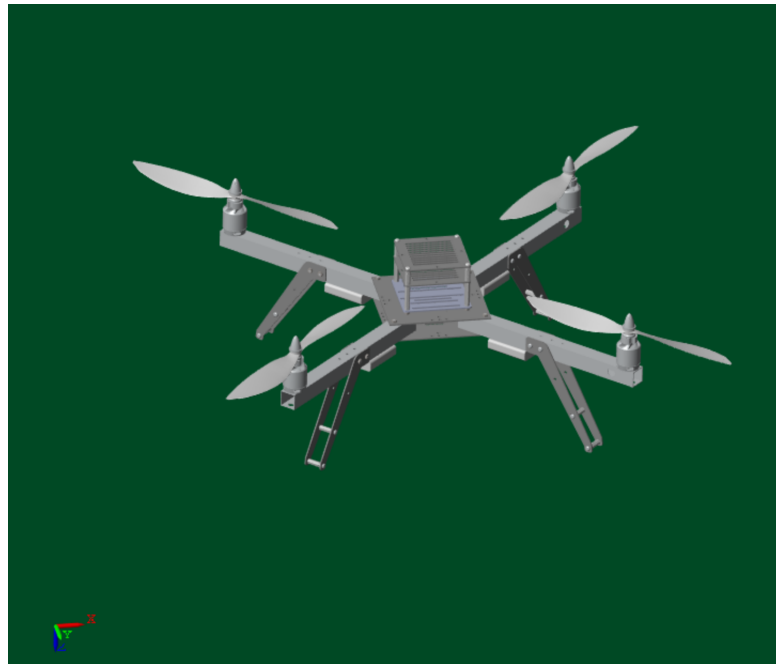
Figure 3.4: Simscape-multibody 3D model of a quadrotor UAV
