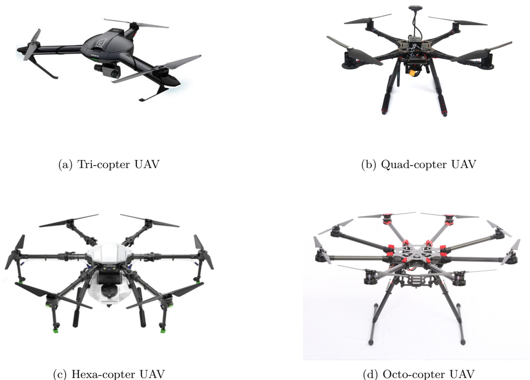
Figure 1.6: Examples of tri-copter UAV, quad-copter UAV, hexa-copter UAV and octo-copter UAV .
