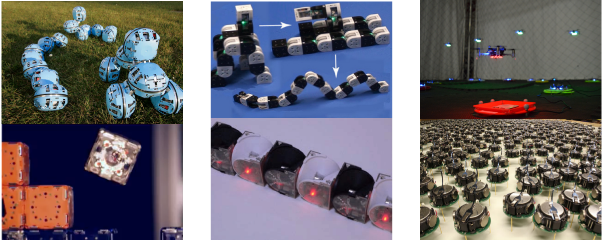
(a) Example of two lattice implementations. Top: ATRON [206]. Bottom: M-Blocks [246].
