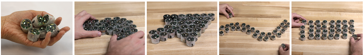
Figure 2.16: Application examples for Zooids [159], a swarm implementation from HCI. Zooids can, e.g., display objects and shapes by acting as physical pixels or communicate user input by acting as physical controllers.
