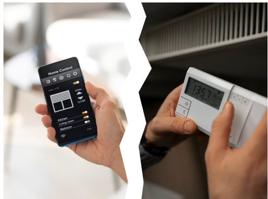
(b) GUI and TUI thermostat controls.
