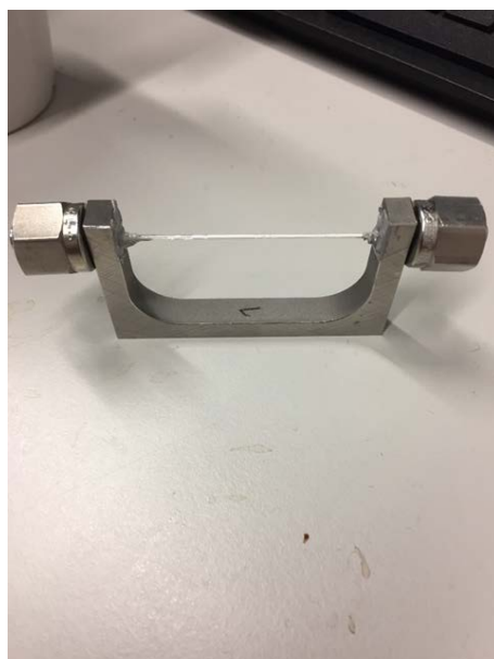
Figure 3. Experimental setup used for in-situ XAS measurements.
