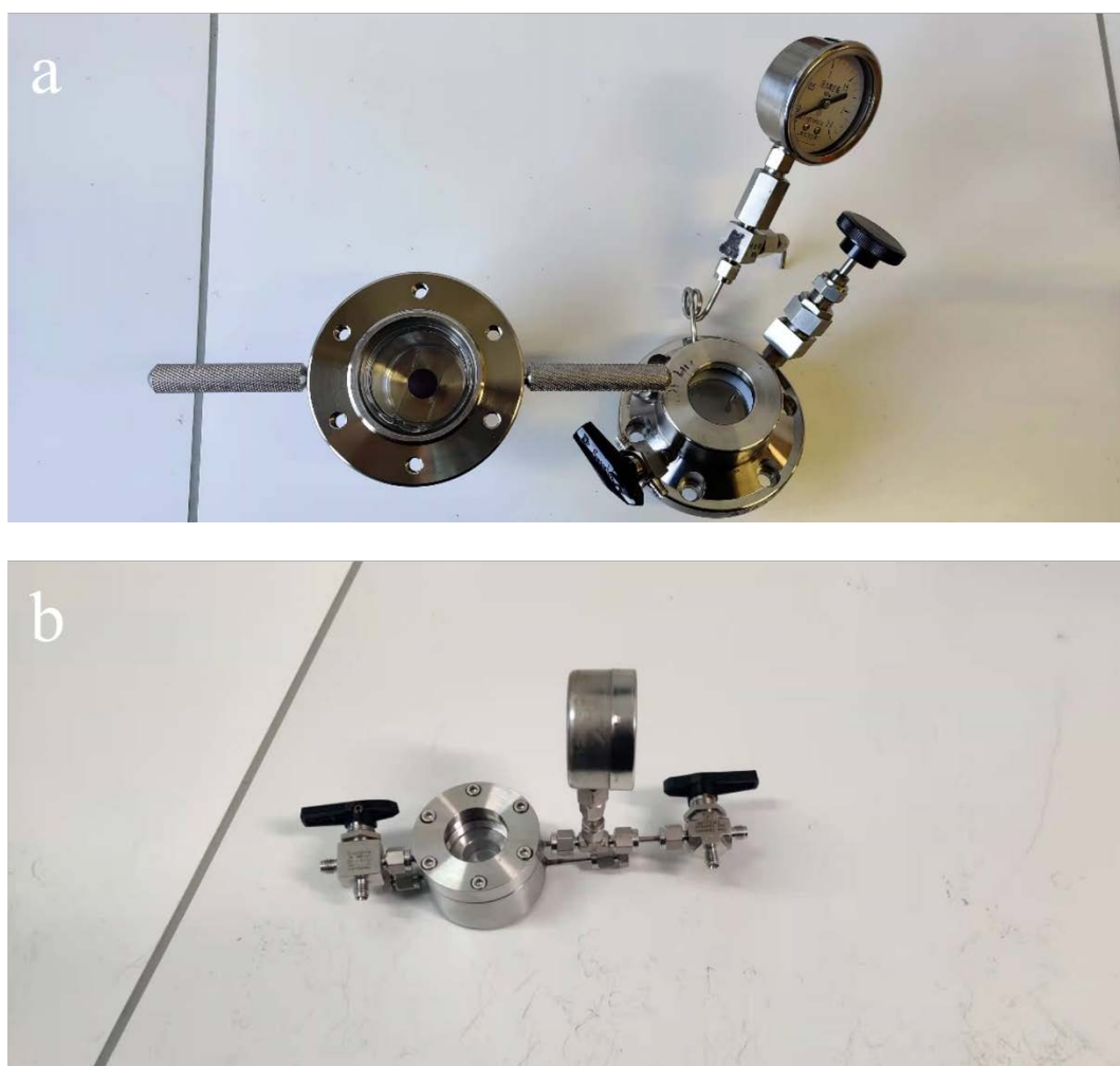
Figure 4. Picture of (a) commercial batch reactor and (b) home-made flow reactor
