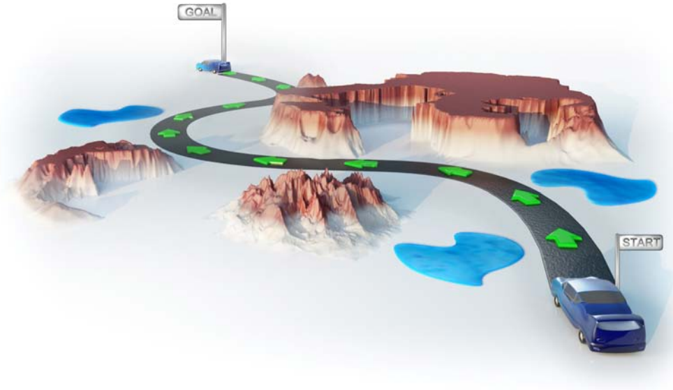
Figure 2.1: Motion planning concept: Finding a collision free path between an initial and final configurations.
