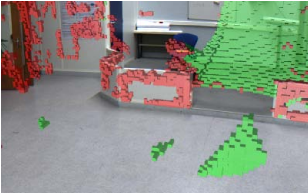
Figure 5.2: The robotic lab in LAAS-CNRS which is modeled based on this approach. Red and green voxels (cube) represent occupied and unknown volumes respectively in the model. The work space is modeled with 3D voxels of 5\text{cm} \times 5\text{cm} \times 5\text{cm} . Notice that this model is the result of several stereo-images taken from different points.
