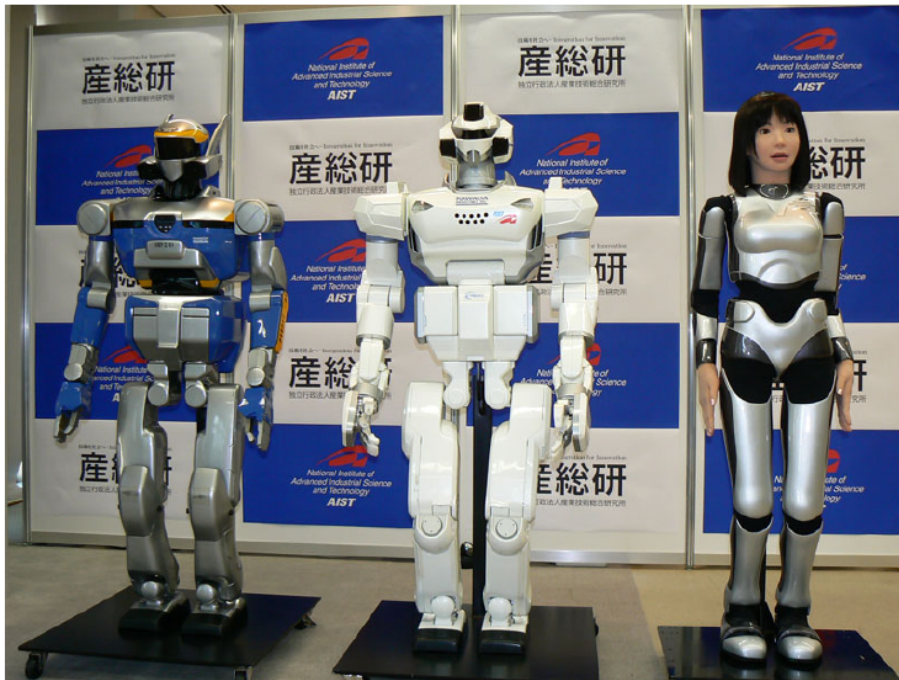
Figure 1.1: HRP platforms. Right to left: HRP2, HRP3 and the last humanoid HRP4.
