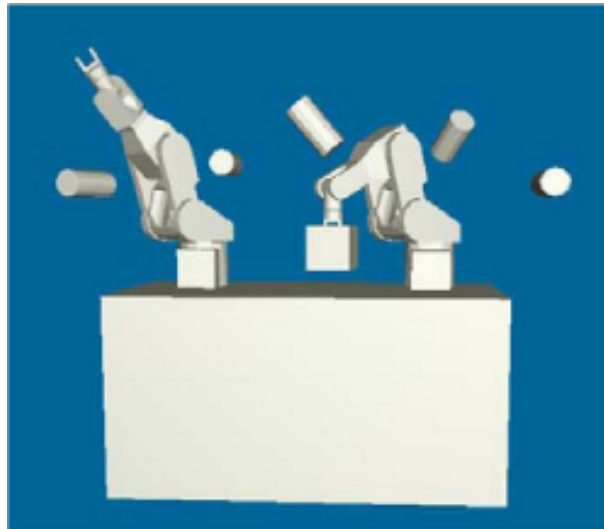
Figure 3.11: From [45]: Path planning for a dual-manipulators system with 12 DOFs in changing environments.
