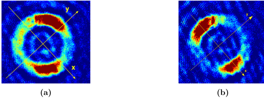
Figure 3.5 — Representation of the change in parameters for the in-plane antennas. Fig.a is what happens when \delta_\phi is not well tuned and the axis between the 2 spots is not along the circle diameter. Fig.b shows a picture where \delta_B is not well tuned, hence having two spots of atoms.
