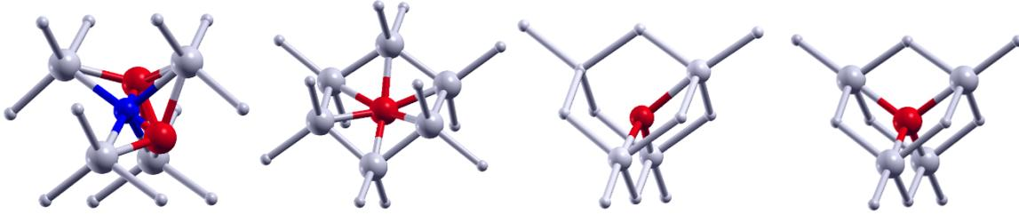
**Figure 1.11:** *Different interstitials configurations. Blue balls indicate a missing atom and red balls an additional atom. From left to right :  $I_{dumbel}^0$ ,  $I_{hex}^0$ ,  $I_{dhex}^1$  and  $I_{tet}^{+2}$  interstitial configurations. (pictures from M3 Team in LAAS-CNRS, not published)*
