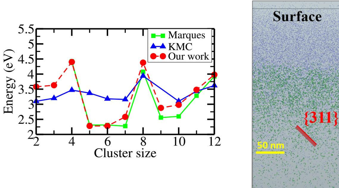
**Figure 4.27:** (Left) Activation energies for interstitial emission depending on the SMICs size (Right) Predicted  $\{311\}$  in KMC using the calibration presented on the left.
