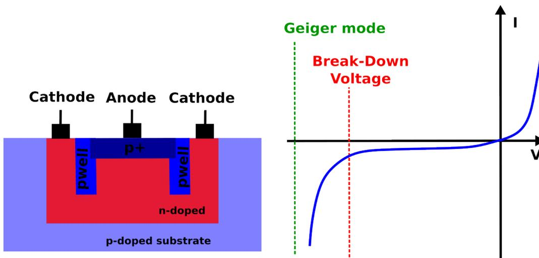
Figure 1.5: (Left) Architecture of a SPAD pixel - (Right) Schematic of the functioning of a SPAD as a function of the applied voltage bias.
