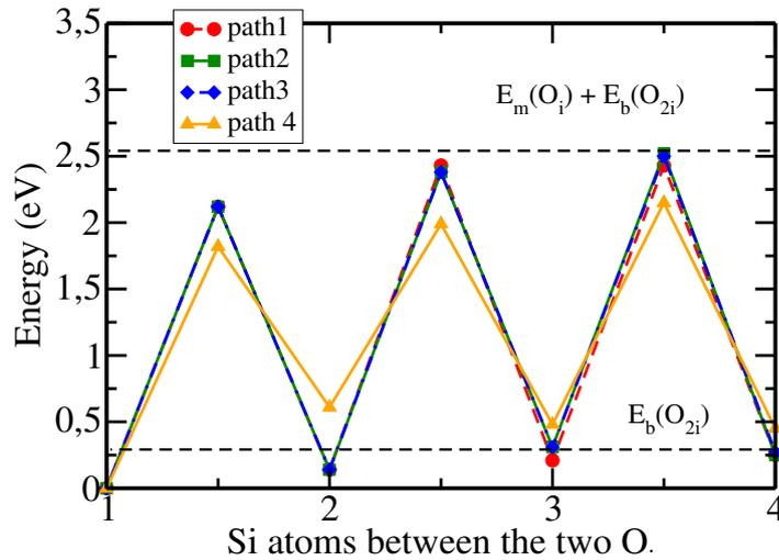
**Figure 3.23:**  $\text{O}_{2i}$  dissociation energies for saddle structures and intermediate stable structures calculated with ARTn. Path 1, 2, 3 start with the  $\text{O}_{2i} \rightarrow 2\text{O}$ . Path 4 is  $2P \rightarrow 3PP \rightarrow 4PPP$ .
