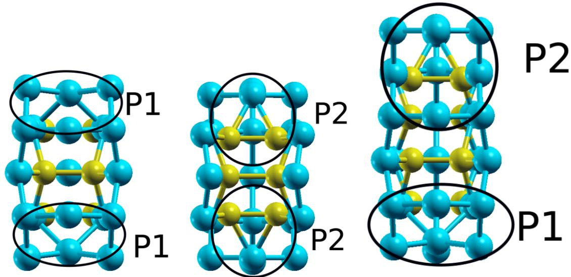
**Figure 4.30:** The different possibilities to form  $I_3$  chain-like clusters after MD relaxations. (Left)  $I_3$  with a P1 extremity (Middle)  $I_3$  with a P2 extremity (Right)  $I_4$  with a P1 and P2 extremity.
