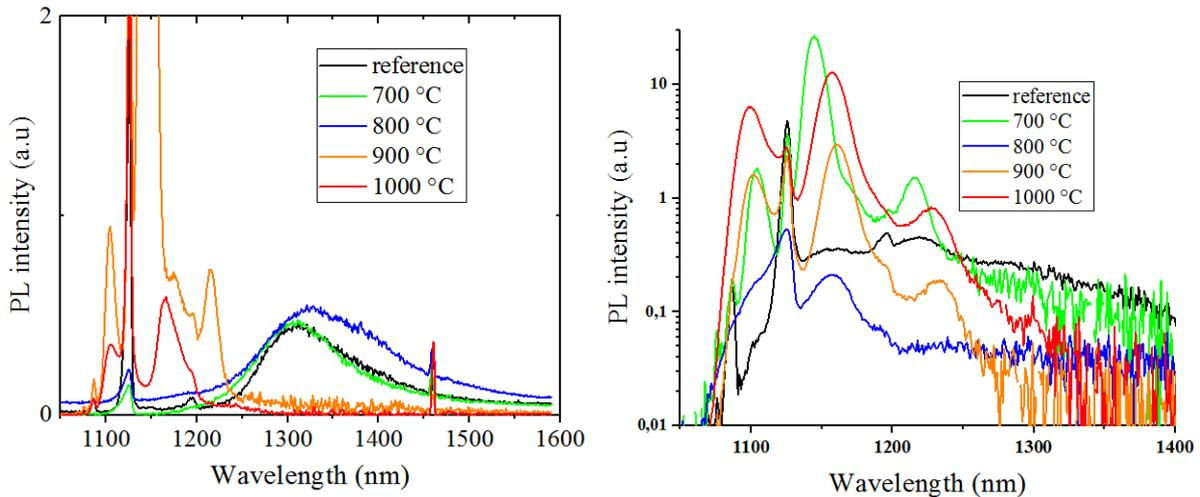
**Figure 4.17:** Photoluminescence spectra after additional annealing for the wafer initially implanted at 150 °C (Left) and 500 °C (Right).
