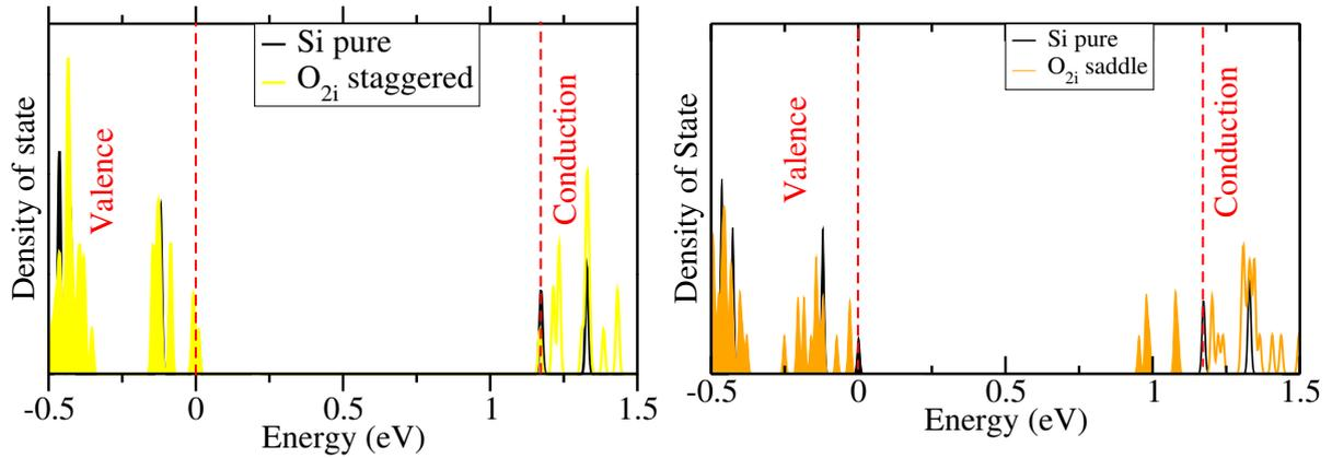
Figure 3.15: DOS for  $\text{O}_{2i}$  stable structure and migration saddle point structure.
