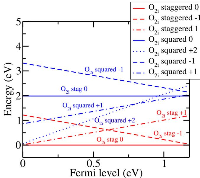
**Figure 3.4:** O<sub>2i</sub> formation energies calculated using HSE formalism in neutral, +1 and +2 charge states for squared configuration and in neutral, -1 and +1 charge states in staggered configurations.
