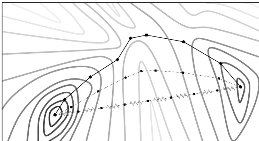
**Figure 2.8:** Illustration of a calculation between two atomic configurations using NEB calculation. The lines in the background represent the isopotential surfaces of the PES. The lines connected by squares represent the intermediate configurations at different cycles of the calculation.
