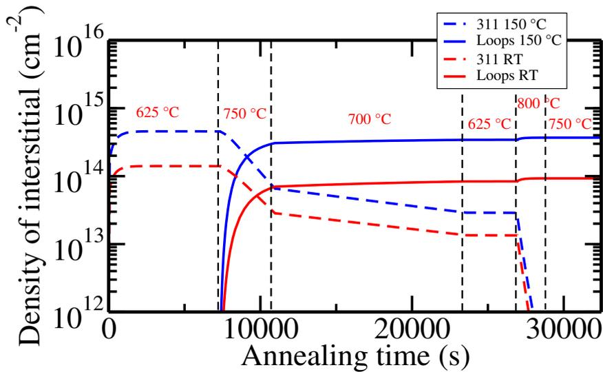
**Figure 4.24:** Number of I trapped in DLs and  $\{311\}$  defects using the hybrid approach combining KMC and continuum model after implantation at RT (red) and at 150 °C (blue).
