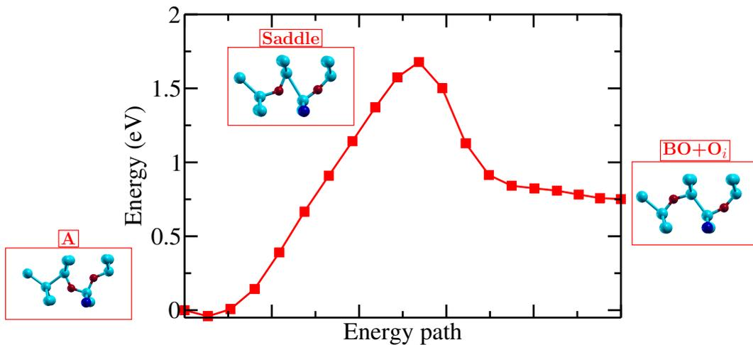
*Figure 3.36: NEB calculations of  $B_s O_{2i}$  dissociation with  $O_i$  going away from  $BO_i$  complex.*
