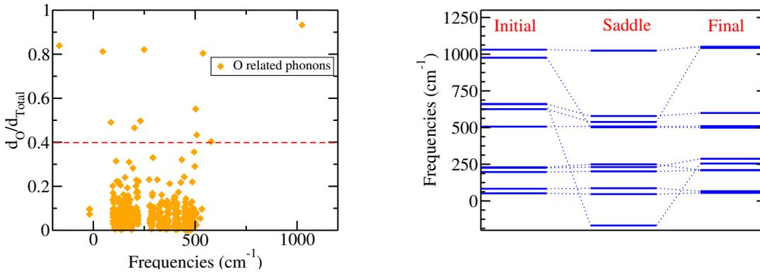
**Figure 3.32:** (Left) Part of oxygen displacement in the phonons of  $\text{O}_{2i}$  to 2-P saddle point. (Right) Projection of the phonons related to oxygen (upon the dotted red line in the left figure) on the phonons of  $\text{O}_{2i}$  and 2-P.
