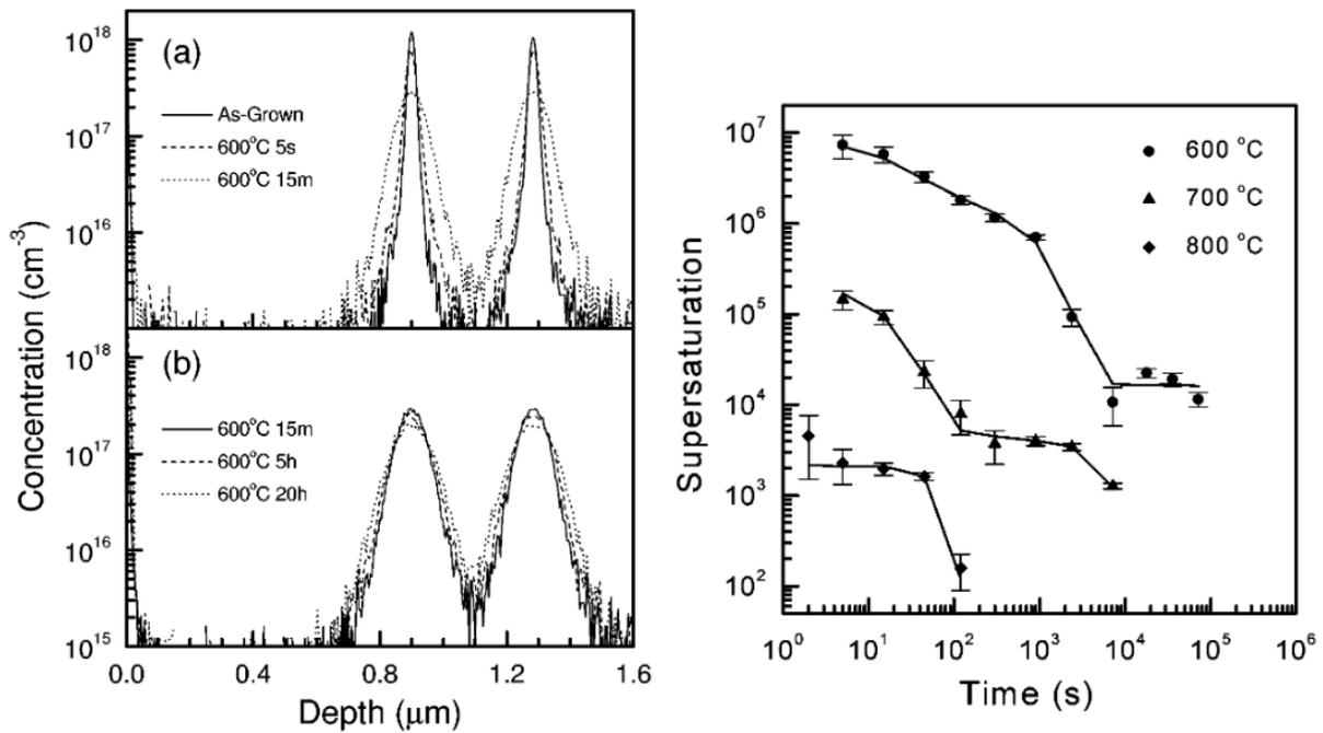
**Figure 2.11:** (Left) Boron marker scattering after  $\text{Si}^+$  implantation as a function of annealing time [29] (Right) Extraction of supersaturation using Boron marker diffusion as a function of temperature and annealing time.
