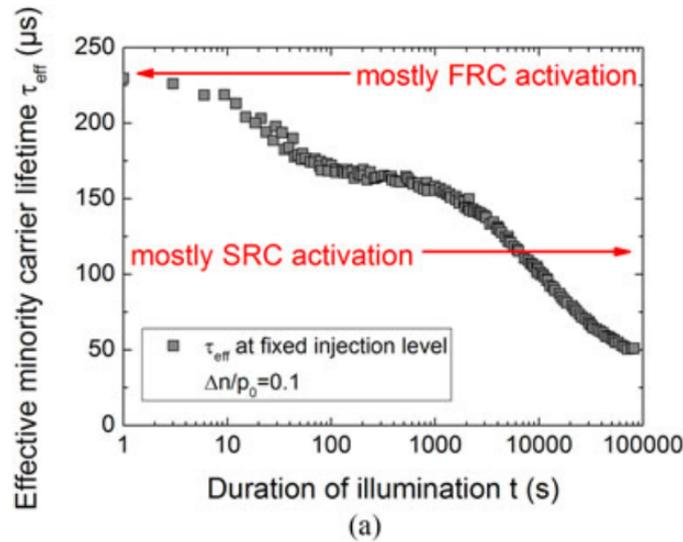
**Figure 1.19:** Evolution of the minority carrier lifetime as a function of time under illumination [41]. Two regimes can be observed.
