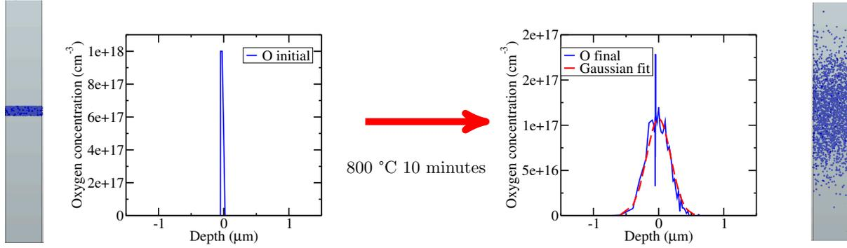
**Figure 3.17:** Methodology to extract the diffusivity from KMC simulations.
