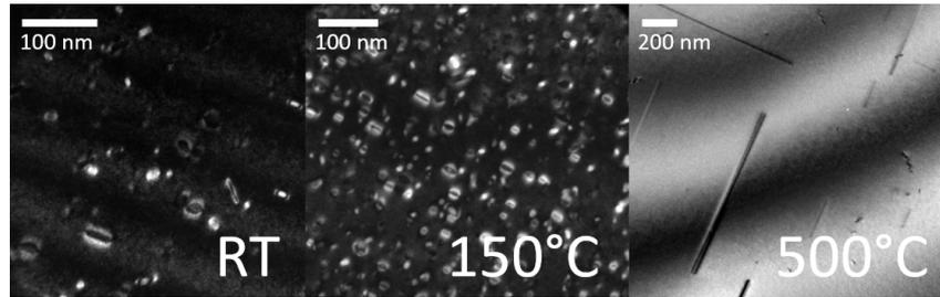
**Figure 4.12:** Plan view TEM micrographs taken from samples implanted with As (cf. Table 4.4 for implant details) and annealed according to Table 4.5. The As implants were carried out at different temperatures: room temperature (left), 150°C (center) and 500°C (right).
