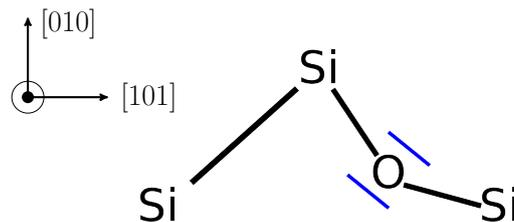
**Figure 3.26:** Diagram of the valence electrons of oxygen  $O_i$ . Two of them participate to Si-O bond and two other electrons are in non-bonding doublet.
