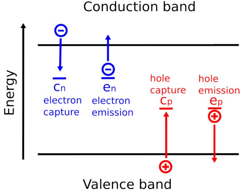
**Figure 1.9:** Capture and emission of holes and electrons by a trap in the silicon gap.
