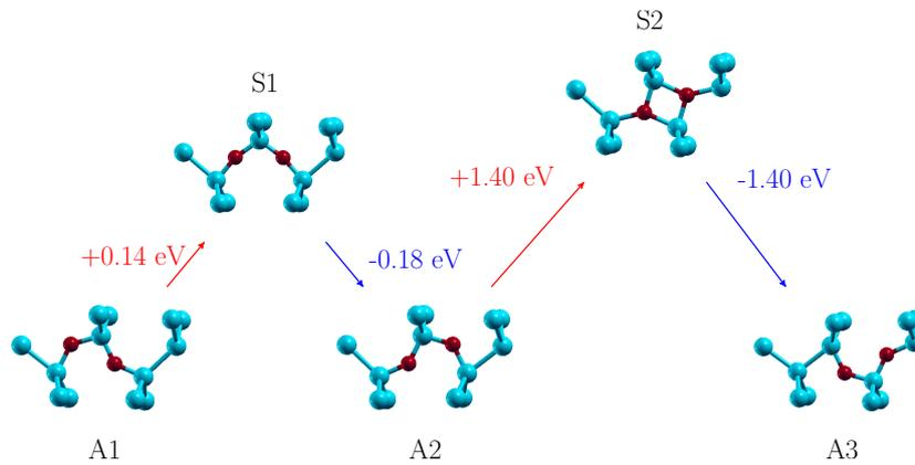
**Figure 3.13:** *O<sub>2i</sub> migration path between two staggered configurations. Activation barriers are given in eV obtained for PBE calculations.*
