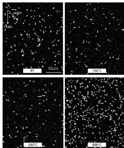
**Figure 1.20:** Photoluminescence imaging of wafers implanted at different temperatures (RT,  $150^{\circ}\text{C}$ ,  $300^{\circ}\text{C}$  and  $500^{\circ}\text{C}$ ) then annealed at  $950^{\circ}\text{C}$  for 3 minutes from . Extended defects are visible in white on the images.
