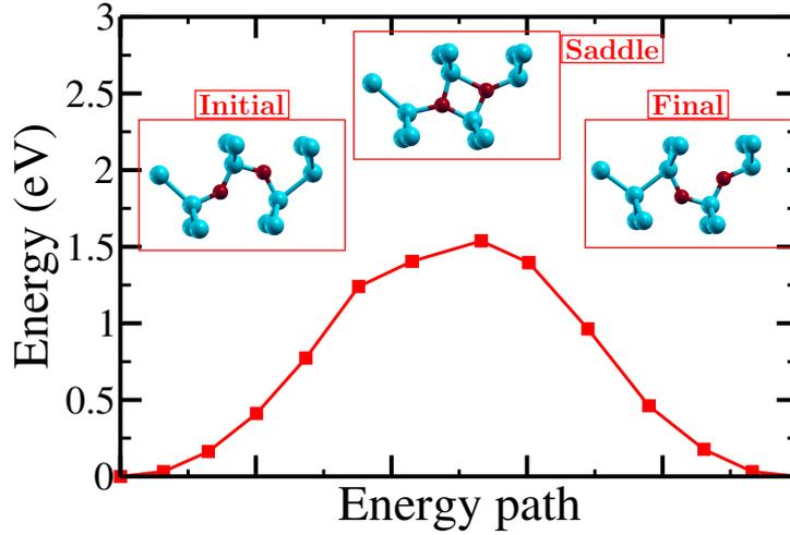
Figure 3.14:  $\text{O}_{2i}$  migration path determined with NEB method for PBE calculations.
