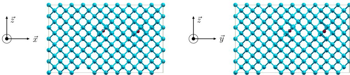
**Figure 3.24:** (Left) 600 atoms silicon cell used for the calculation (Right) Saddle and intermediate structures obtained with ARTn for the  $\text{O}_{2i}$  dissociation in the (101) direction.
