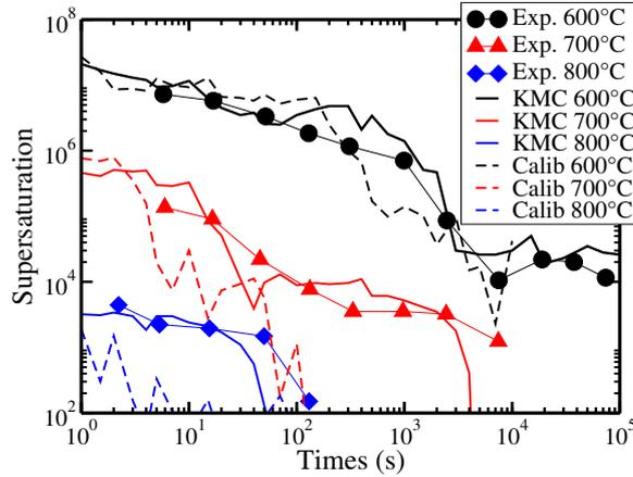
**Figure 4.29:** Comparison of supersaturation extracted from [25] experiments (exp in the legend) and predicted by the KMC using the default implementation (KMC in the legend) and the calibrated energies on the As implementations (calib in the legend).
