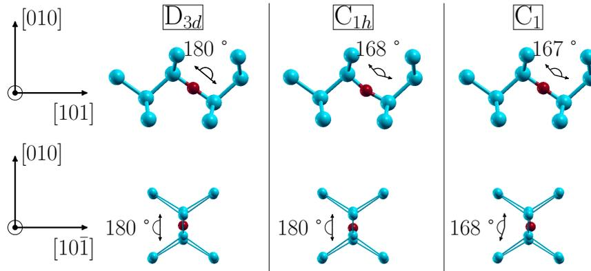
**Figure 3.1:** Different  $O_i$  configurations relaxed with *ab initio* calculations, from left to right:  $D_{3d}$ ,  $C_{1h}$  and  $C_1$ . The configurations are represented in a  $(101)$  plane (top) and in its orthogonal plane  $(10\bar{1})$  (bottom).
