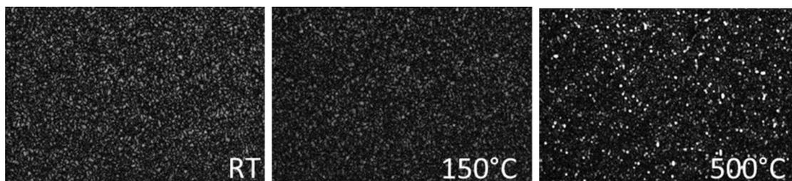
**Figure 4.13:** PL imaging maps (120x175  $\mu\text{m}$  area) taken from samples implanted with As (cf. Table 4.4 for implant details) and annealed according to Table 4.5. The As implants were carried out at different temperatures: room temperature (left), 150°C (center) and 500°C (right).
