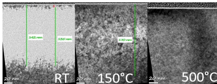
**Figure 4.10:** Cross section TEM micrographs taken from samples implanted with As (cf. Table 4.4 for implant details) at different implant temperatures: room temperature (left),  $150^{\circ}\text{C}$  (center) and  $500^{\circ}\text{C}$  (right).
