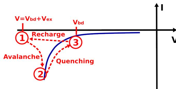
**Figure 1.7:** Cycle of operation of a SPAD type pixel during the detection of a photon.
