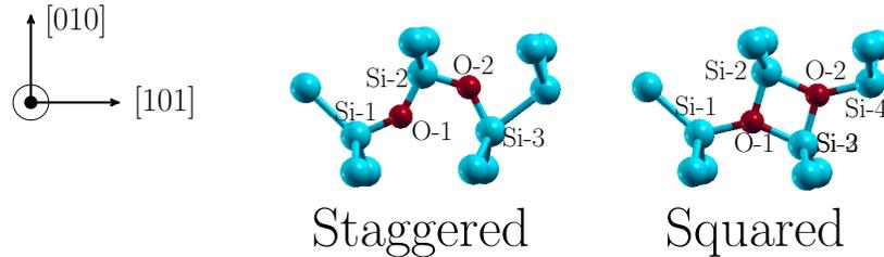
**Figure 3.3:**  $O_{2i}$  configurations: staggered (left) and squared (right) in a (101) plane from *ab initio* simulations.
