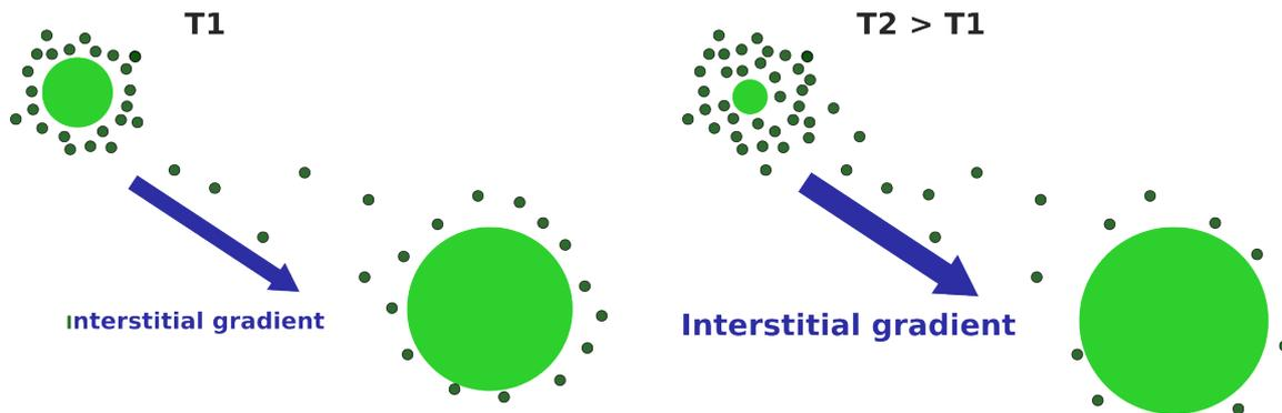
**Figure 1.17:** Ostwald maturation model leading to the formation of more and more extended and fewer defects during annealing.
