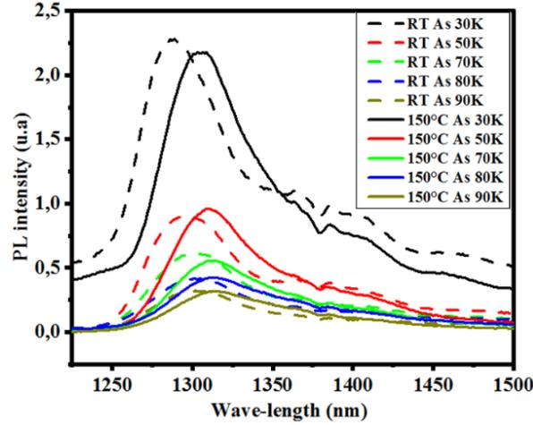
**Figure 4.15:** PL spectra acquired at different temperatures from samples implanted with As (cf. Table 4.4 for implant details) and annealed according to Table 4.5. The As implants were carried out at different temperatures: room temperature (left), 150°C (left) and 500°C (right).
