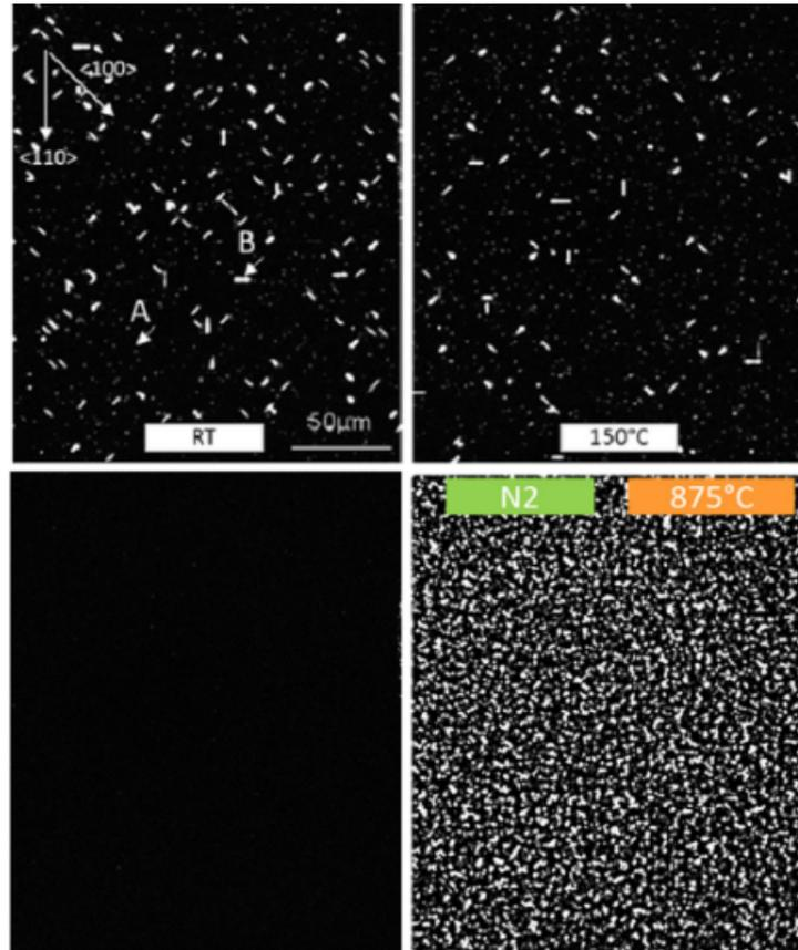
**Figure 4.6:** Photoluminescence imaging maps taken from samples implanted with high-energy  $P$  ions with different conditions (cf. Table 4.2). Top left: Sample Ph 2. Top right: Sample Ph 3. Bottom left: Sample Ph 12. Bottom right: Sample Ph 18.
