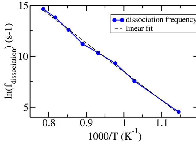
**Figure 3.38:** Logarithm of the dissociation frequency in the off-lattice KMC depending on the temperature using an intermediate points in the O<sub>2i</sub> dissociation path (averaged on 20 simulations).
