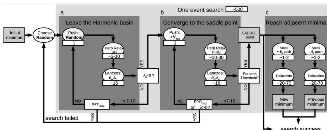
**Figure 2.9:** ARTn working scheme [24] where the three main phases of the algorithm are depicted within the shaded dark gray rectangles. Phase (a) involves escaping from the harmonic basin; phase (b) focuses on converging towards the saddle point; and phase (c) centers on reaching the neighboring minima.
