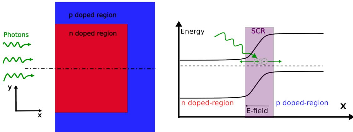
Figure 1.4: Structure of a pixel and its Fermi level along dashed line.
