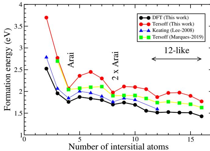
**Figure 4.31:** Comparison of the interstitial formation energies of SMICs from [22] and [23] works and the energies calculated in this thesis using the coupled MD - DFT strategy.
