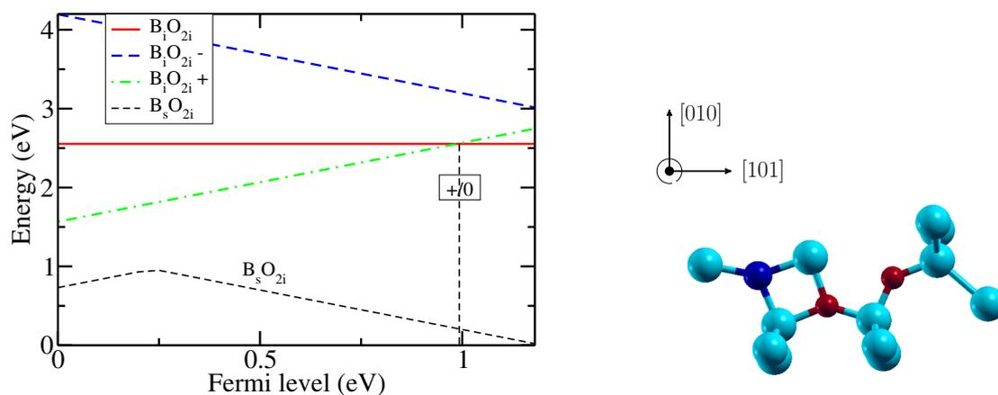
**Figure 3.8:**  $B_i\text{O}_{2i}$  formation energy compared to  $B_s\text{O}_{2i}$  formation energy calculated with HSE.
