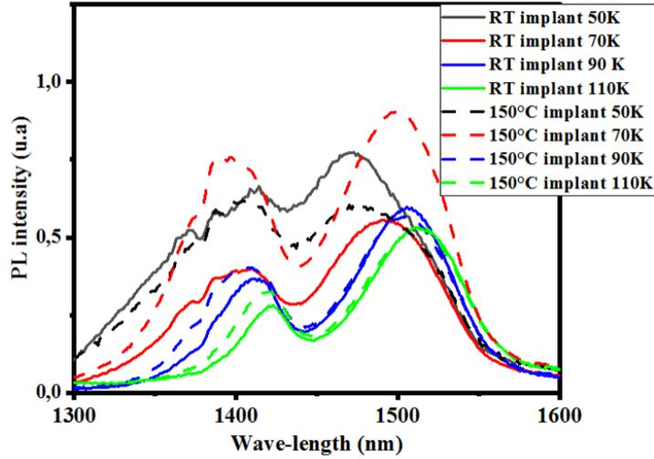
**Figure 4.8:** PL spectra acquired at different temperatures from samples Ph2 and Ph3 (cf. Table 4.2) implanted with P at different temperatures (RT and  $150^\circ\text{C}$  respectively).
