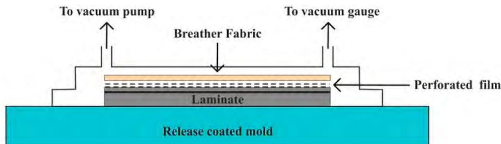
Figure 1.15: Vacuum bag molding process.(Rajak et al., 2019)
