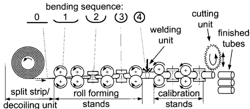
Figure 1.14: Principle of tube roll forming process. (Groche and v. Breitenbach, 2008)
