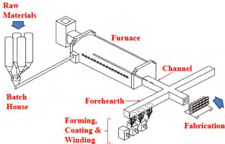
Figure 1.3: Glass fiber manufacturing principle. (Stickel and Nagarajan, 2012)
