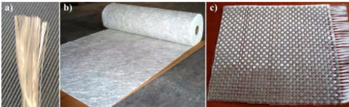
Figure 1.4: Examples of available forms of fiber reinforcements (Correia, 2023).
