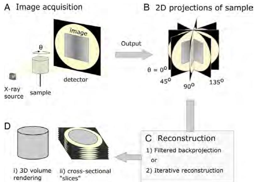
Figure 1.40: Diagrammatic representation of X-ray micro-computed tomography workflow. (O'Sullivan et al., 2018)
