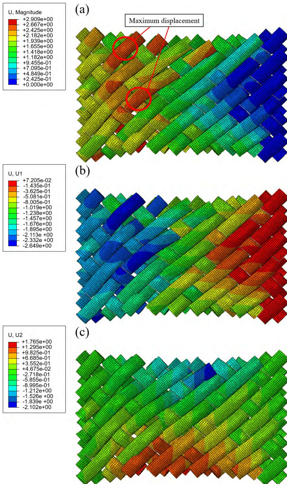
Figure 4.25: Displacement field resulting from the simulation of a "mini" bias test in Abaqus: (a) displacement magnitude; (b) and (c) are respectively the components of the displacement field in the horizontal and vertical axes (along X and Y, respectively).
