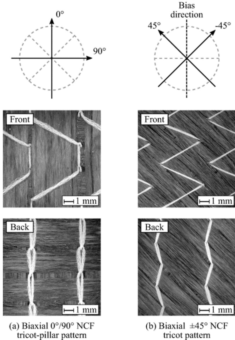
Figure 1.27: Example of two representative biaxial NCF configurations with their respective layer orientations. (Colin et al., 2020)
