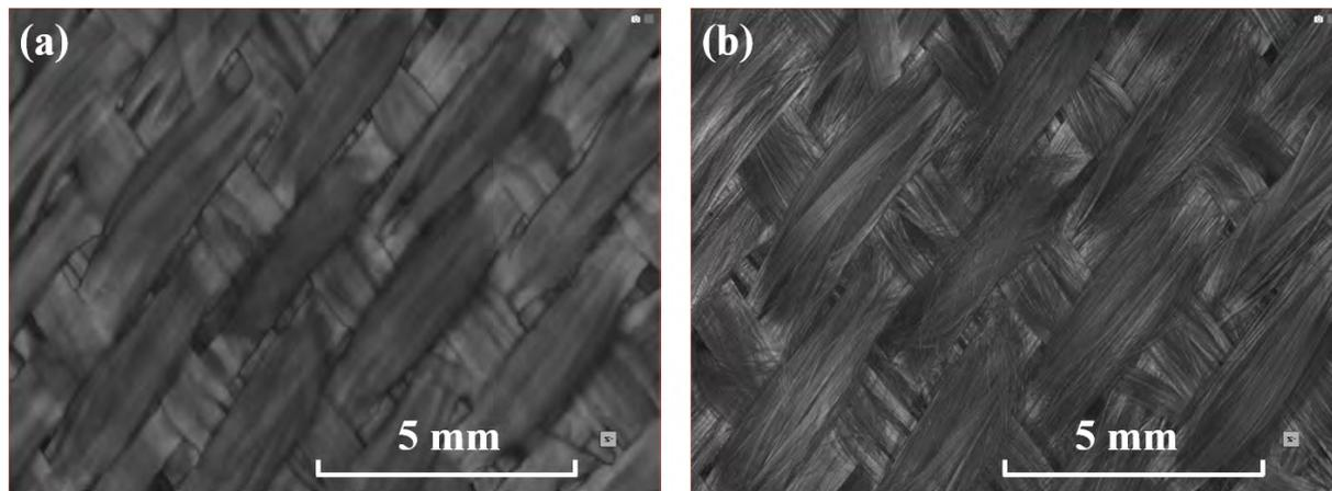
Figure 4.6: Qualitative comparison of volume images reconstructed at resolutions of  $47.5 \mu\text{m}/\text{vx}$  (a) and  $10.3 \mu\text{m}/\text{vx}$  (b) in a common zone. It shows that tomography at the higher resolution reveals the architecture, and even the fibers arrangement, much better. As a reminder, the glass fibers diameter is around  $10 \mu\text{m}$ .
