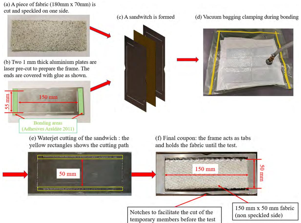
Figure 2.3: Proposed bias test specimen preparation procedure. An aluminum frame is added to the fabric piece so that the warp and weft remain well oriented at  $\pm 45^\circ$  throughout the test preparation. The end portions will then serve as tabs during the test.
