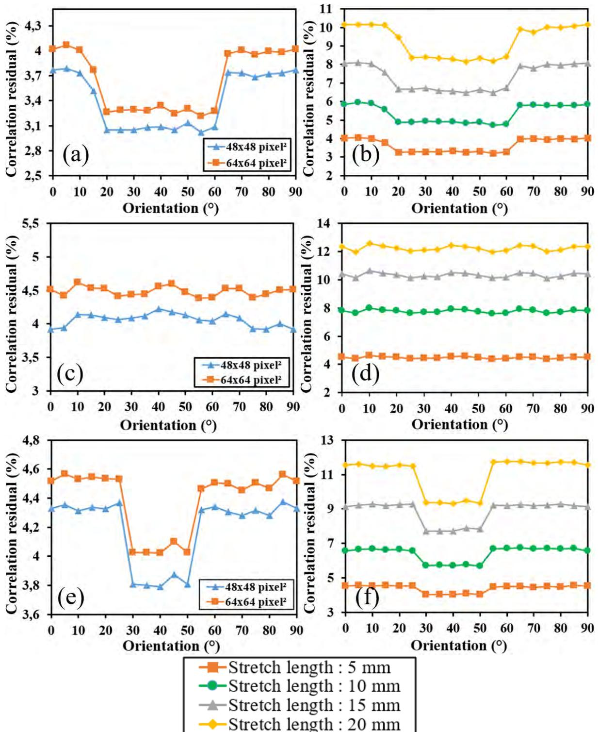
Figure 2.12: Evolution of the standard deviation of the overall residuals  $R$  as a function of the relative mesh orientation/tensile direction  $\theta$  for a glass fabric sample ((a) and (b)), a carbon fabric sample ((c) and (d)), and a C/PPS fabric sample ((e) and (f)).
