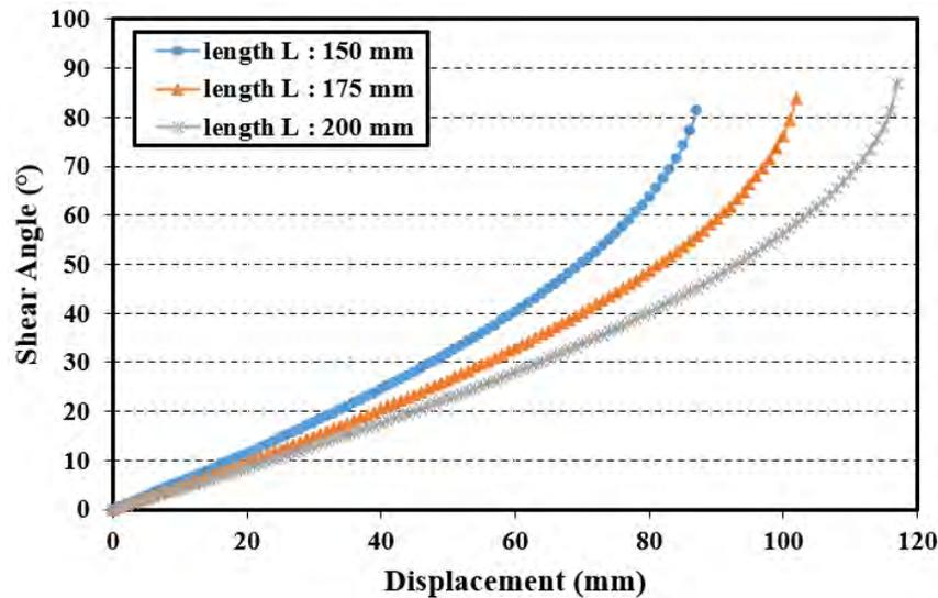
Figure 1.24: Theoretical shear angle obtained from the formula 1.2.
