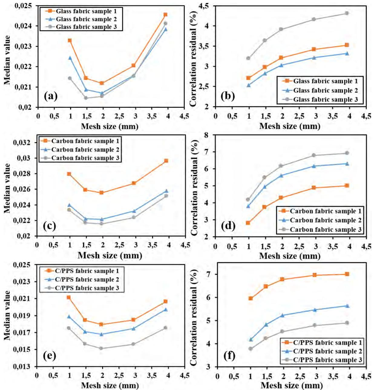
Figure 2.10: Evolution of MRE, the median random error (left-hand column), and of  $R$ , the correlation residuals (right-hand column), as a function of the mesh size. Results for 3 samples of each fabric (from top to bottom: glass, carbon, and C/PPS) are presented. The sample was stretched by 10 mm.
