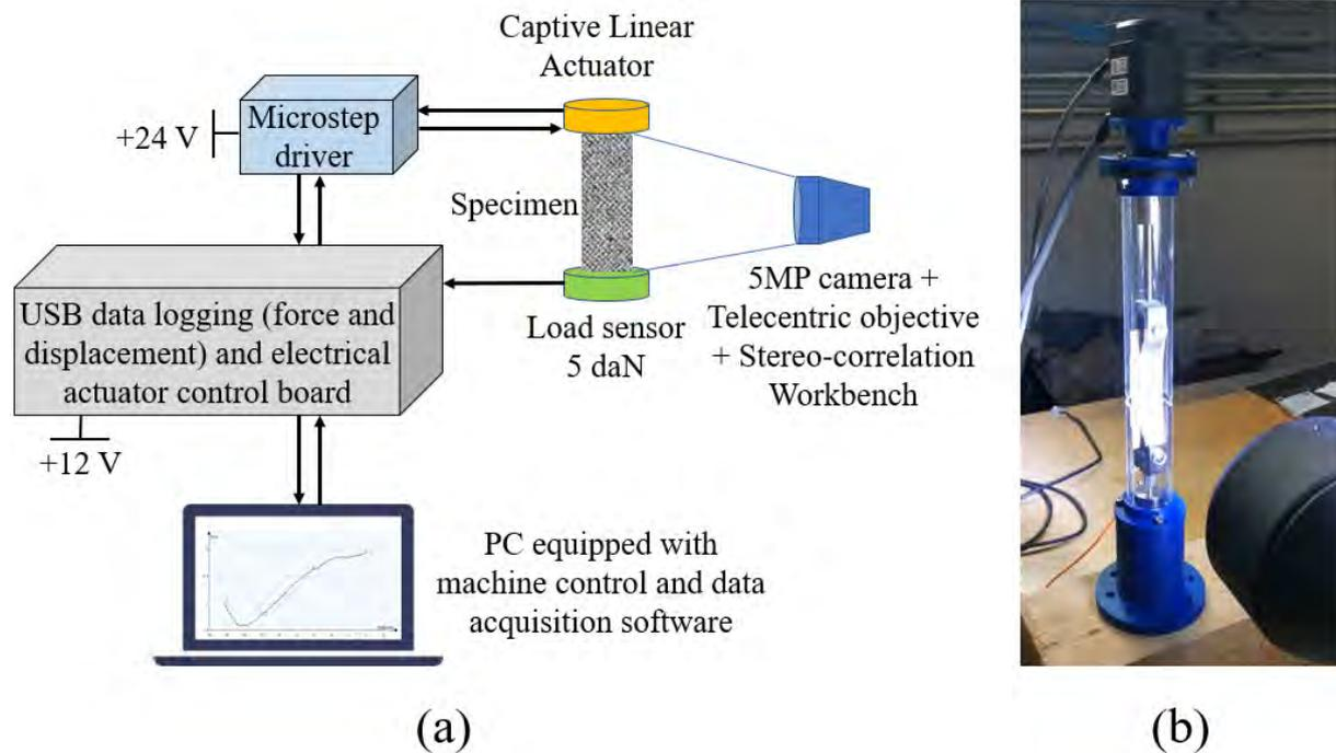
Figure 4.31: Bias extension tests carried out *ex situ* with the miniature tensile machine: (a) experimental setup: the stereo bench, which did not yield convincing results, is not represented; (b) photo of the machine fixed on a table: the side slits made in the PMMA tube allow the fabric to be released (by cutting the side posts of the frame) before the test
