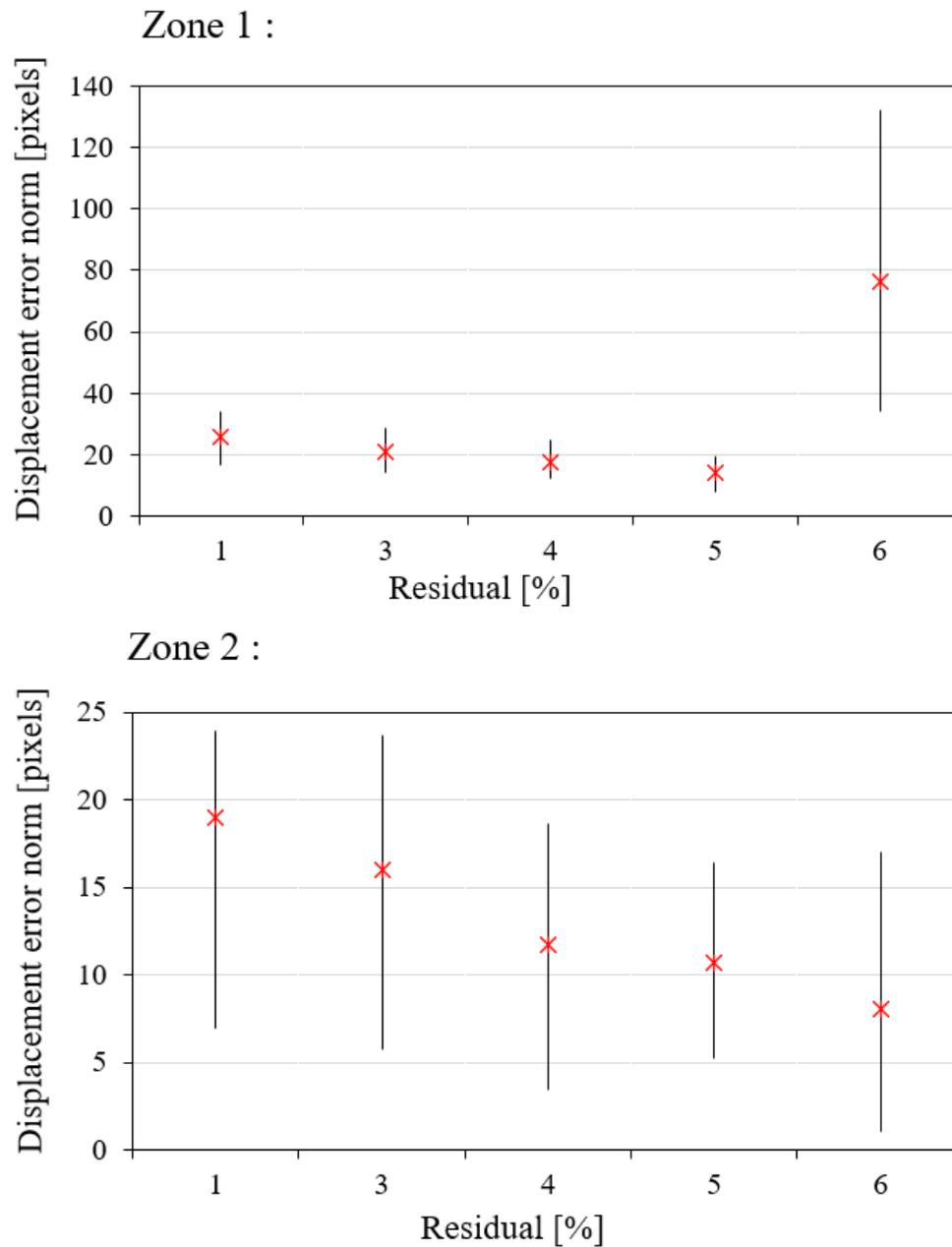
Figure 3.22: The average modulus of the vectors between the mesh nodes and the actual positions for C/PPS fabric sample in zone 1 and zone 2 for different limits.
