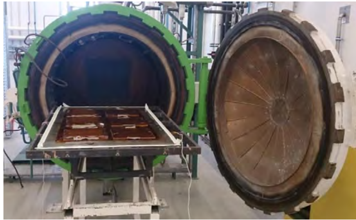
Figure 1.16: Autoclave at Institute Clément ADER - Toulouse (Patou, 2018).
