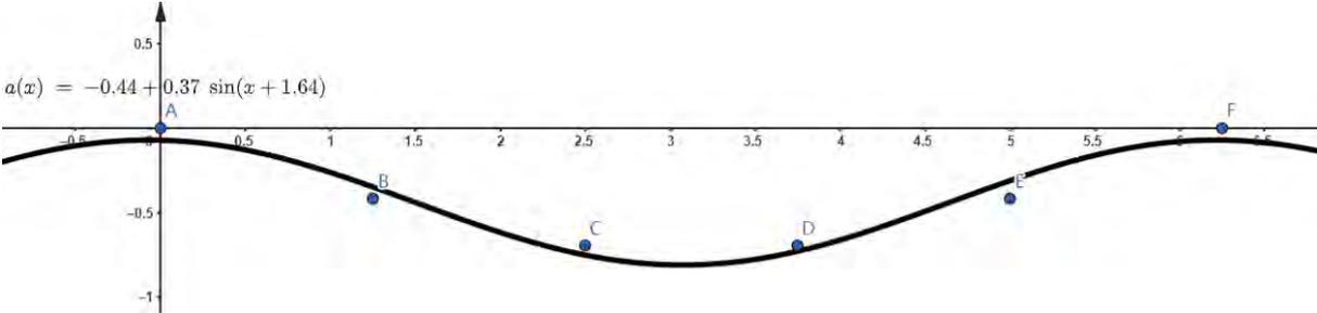
Figure 4.12: The sinusoidal function used here in TexGen to interpolate the yarn path. The blue points correspond to the "master nodes" whose position is estimated from the segmented tomographies.
