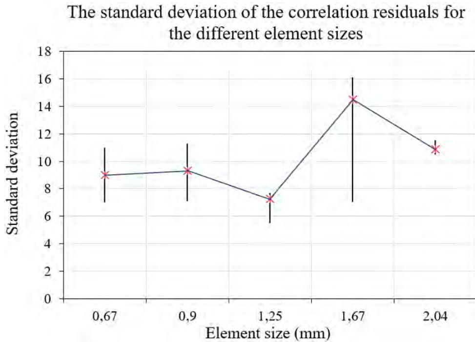
Figure 2.23: Unscaled standard deviation of the displacement errors for different mesh sizes with the same speckles distribution. The red crosses correspond to the displacement norm deviations, while the top and bottom of the bars indicate the displacement deviations along X and Y, respectively.
