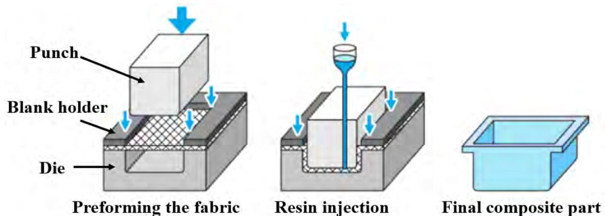
Figure 1.18: Schematics of performing and resin injection molding processes. (Boisse, 2004)
