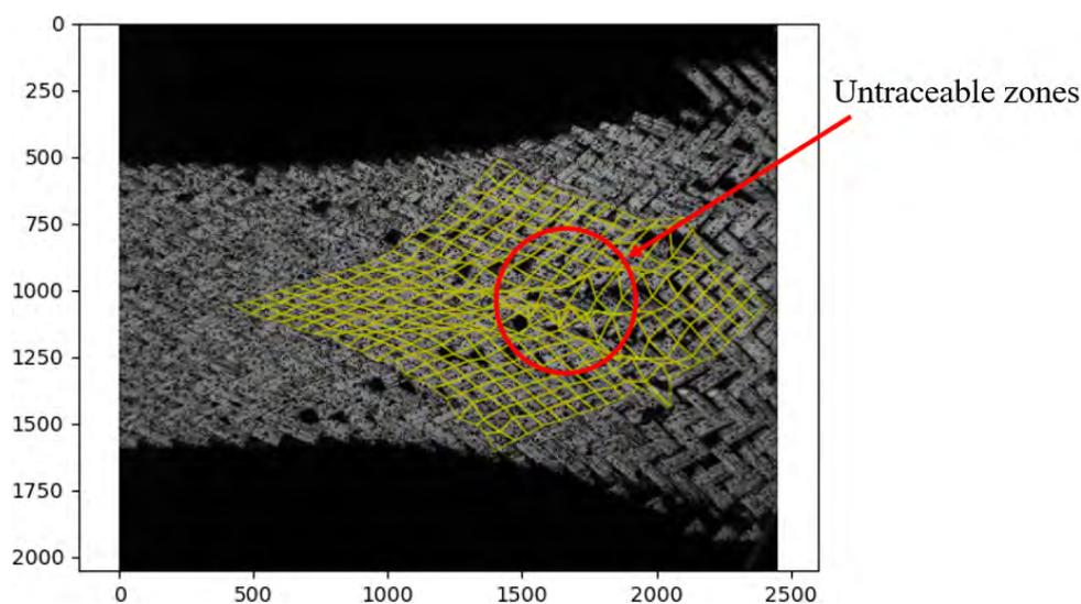
Figure 3.25: Deformed mesh given by incremental FE-DIC with an update constraint based on correlation residuals ( $R < 5\%$ ).
