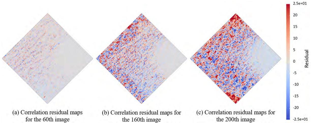
Figure 3.5: Correlation residual maps in the selected ROI for (a) the 60th, (b) the 120th and (c) the 200th image obtained with Pyxel and plotted with ParaView.
