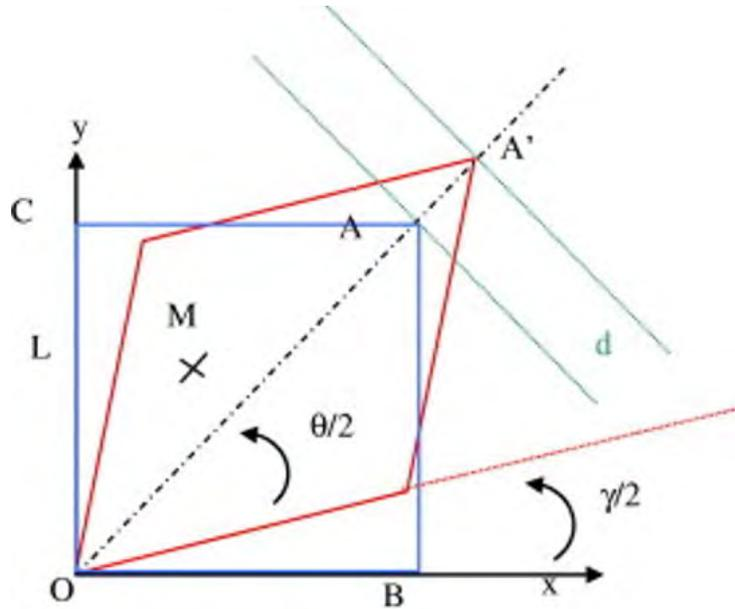
Figure 1.23: Pure shear kinematics. (Launay et al., 2008)
