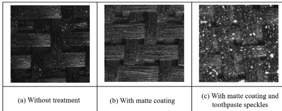
Figure 1.38: Treatment of a carbon fabric with matte coating and toothpaste speckles. (De Luycker, 2009)
