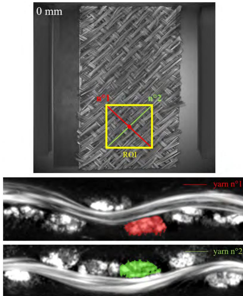
Figure 4.41: The position of the selected cross sections.
