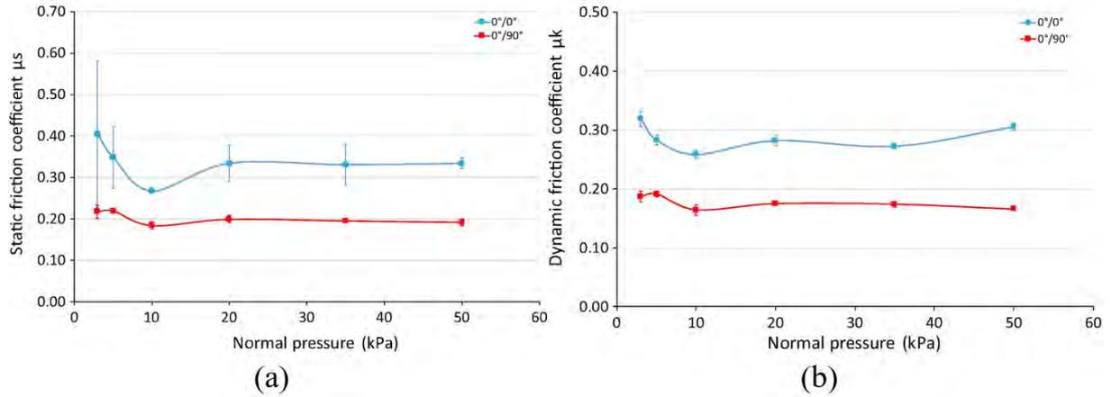
Figure 4.23: Evolution of (a) the static friction coefficient  $\mu_s$ , and (b) the dynamic friction coefficient  $\mu_k$  between yarns versus normal pressure at a speed of 1 mm/sec. Error bars represent standard deviations. These curves are taken from the work of (Montero et al., 2017)
