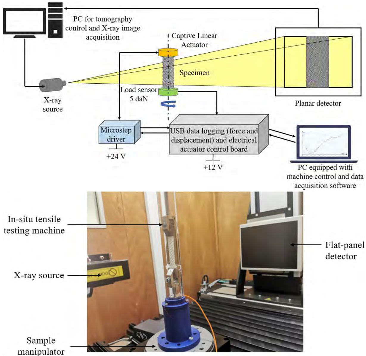
Figure 4.37: Photo showing the *in-situ* traction machine mounted in the ICA tomograph (bottom). A diagram shows the entire system implemented during these tests (top)
