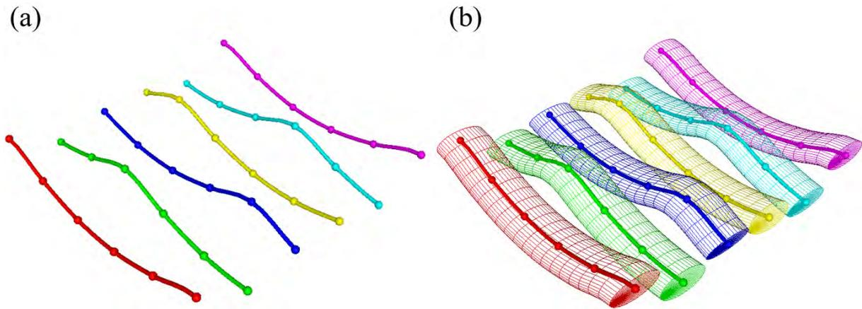
Figure 4.14: (a) Warp yarn paths in the unit cell; (b) CAD model of the warp yarns obtained by sweeping an elliptical section along the paths.
