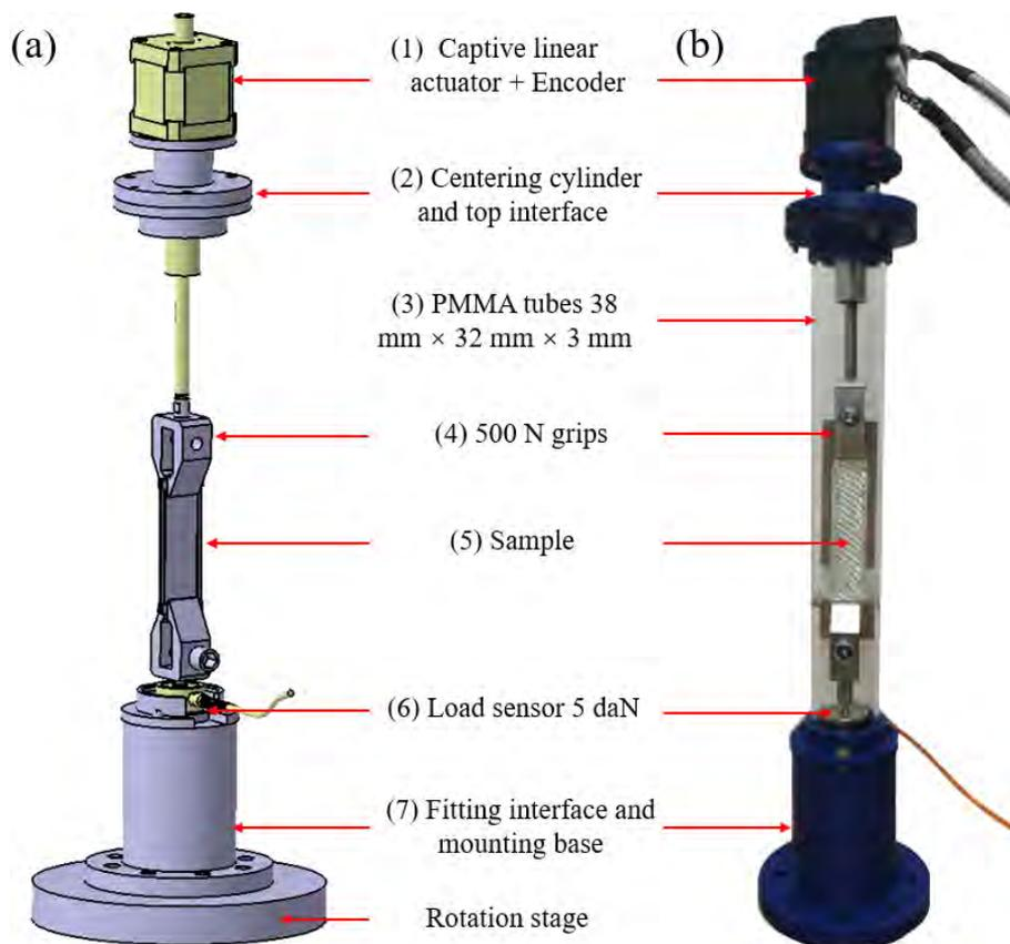
Figure 4.29: *in-situ* tensile machine designed in-house for the purposes of this study: (a) CAD of the machine without the tube and (b) first manufactured version. The main interfaces connecting the commercial parts were obtained by 3D printing.
