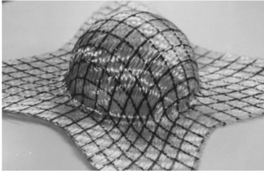
Figure 1.26: Draping of a woven reinforcement on a double-curved surface. (Bai et al., 2022)
