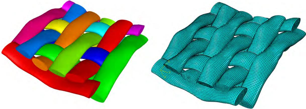
(a) DIB CAD model generated with TexGen      (b) DIB FE model generated with Abaqus
