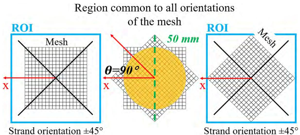
Figure 2.11: A uniform square structured mesh is again used. It is now rotated through an angle  $\theta$  with respect to the tensile direction X. The diagonal of the square mesh matches the width of the useful region. FE DIC measurements are made for angles ranging from  $0^\circ$  to  $90^\circ$ . The correlation residuals  $R$  obtained (standard deviation of correlation residuals) are compared only in the circular region common to all mesh orientations (in yellow).
