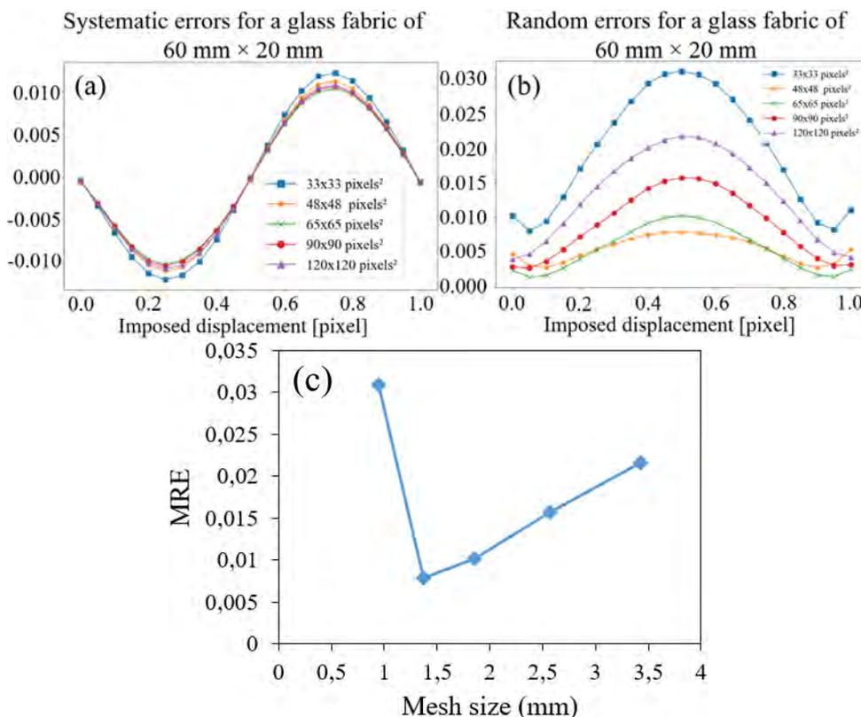
Figure 4.34: Evolution of the ultimate error as a function of mesh size for a 60 mm × 20 mm specimen of speckled glass fabric: evolution of the systematic error (a), the random error  $\sigma_e$  (b) and the median value of the random error, denoted MRE (c).
