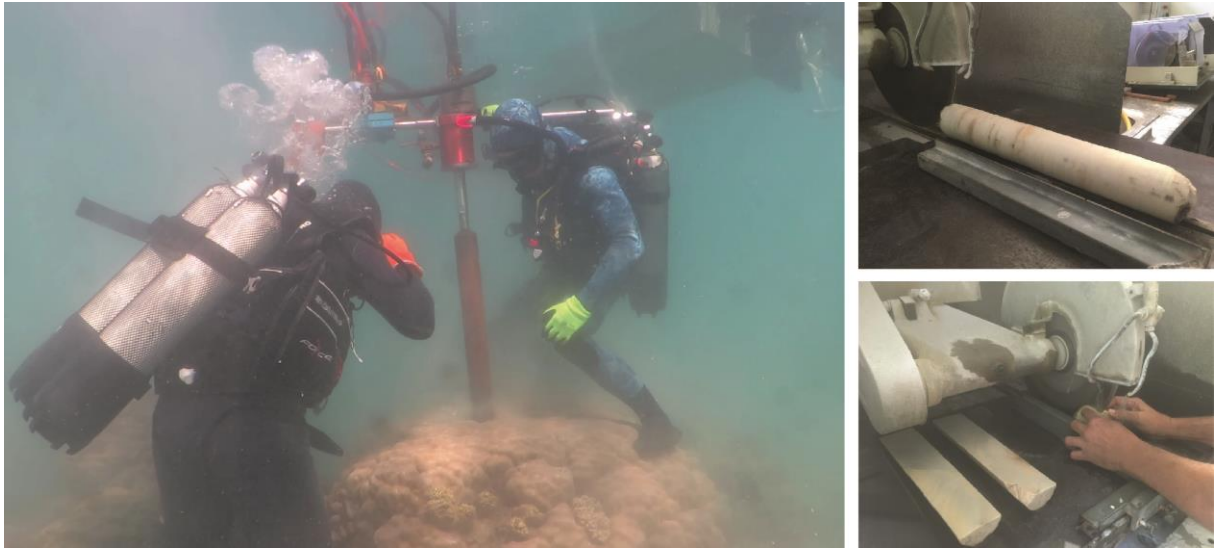
Figure VIII-17 | Drilling and cutting of the two Porites sp. cores from Bouraké and Puen (core length: ~35 cm; core diameter: ~7 cm).
