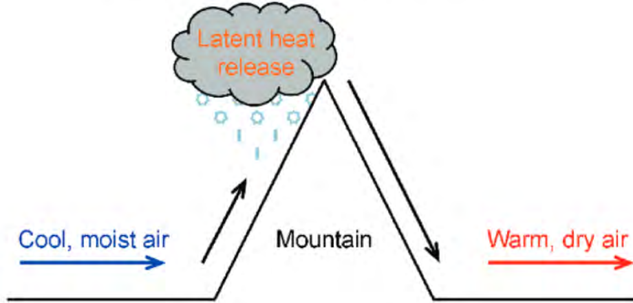
Figure 1.4: Schematic of latent heating and precipitation of winds in the lee of a mountain range. As shown in Elvidge and Renfrew (2016) .
