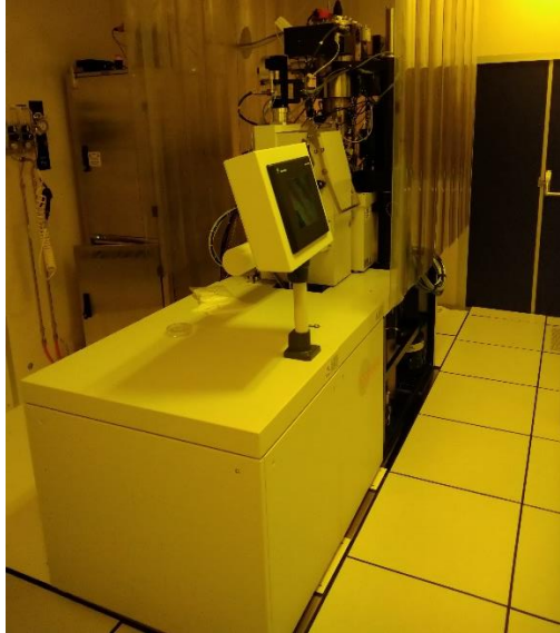
Figure E.5: ebpg 5000Plus E-beam lithography machine from RAITH nanofabrication company.
