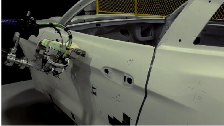
Figure 1.8: Teraview THz sensor integrated to a robot arm measuring the paint thickness on a vehicle [10].
