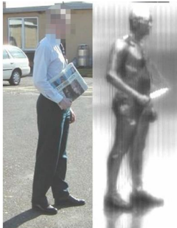
Figure 1.3: Illustration of a detected weapon by THz imagery [4].
