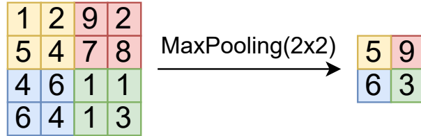
Figure III.4 – Illustration of the processing performed by a max pooling 2 \times 2 layer on an input image.
