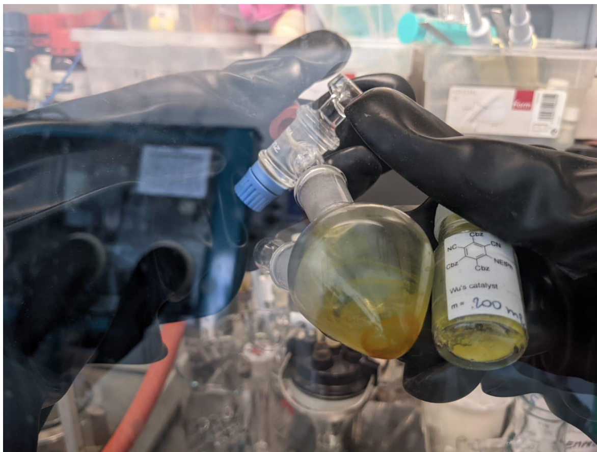
Figure III-74: Photograph of the isolation attempt of 3\text{CzEPAIPN} radical anion (orange, in the flask) next to the starting 3\text{CzEPAIPN} (yellow, in the vial).
