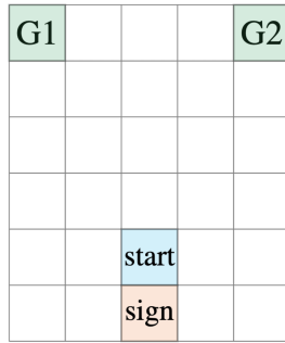
Figure 3.1 – An environment with two tasks: the goal location ( G1 or G2 ) changes at each episode. The sign reveals the location of the goal. Optimal informed policies are shortest paths from start to either G1 or G2 , which never visit the sign. Thompson sampling cannot represent the optimal exploration/exploitation policy (go to the sign first) since going to the sign is not feasible by any informed policy.
