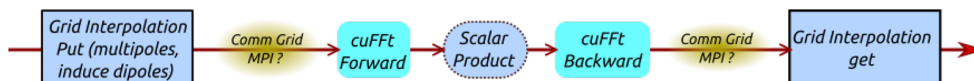
Figure 4. Reciprocal space offload scheme. Charge interpolation and Force interpolation are both written in a single kernel. They are naturally parallel except for the atomic contributions to the grid in the first one. The approach remains the same for data management between host and device as for real space: all data are by default device resident to prevent any sort of useless transfer. Regarding MPI communications, exchanges take place directly between GPUs through interconnection.
