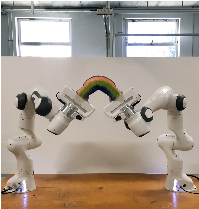
FIGURE 5.6: Our experimental setup with two Franka robots manipulating a foam octagonal cylinder. An overhead 3D camera provides the input for our approach.
