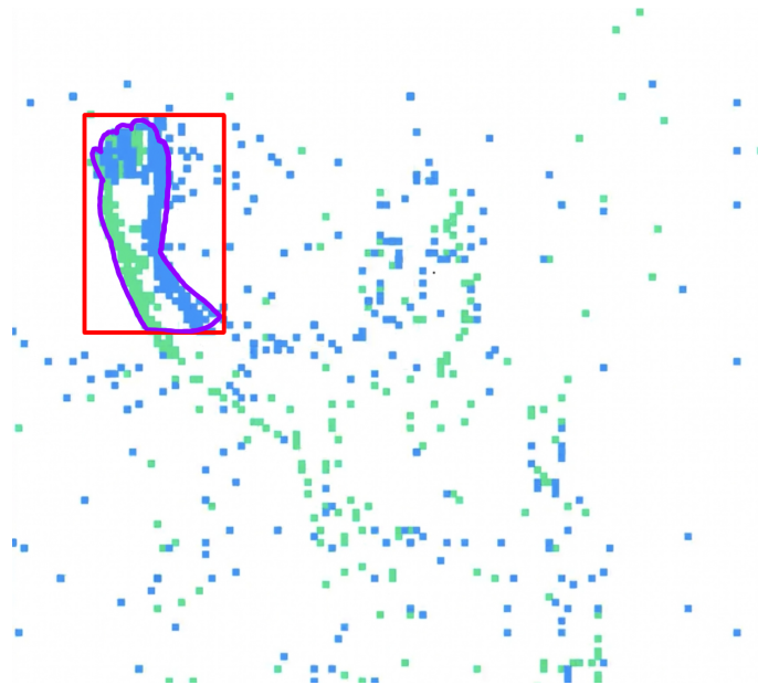
Figure 7.1 – Visual example of the difference between an RoI (outlined in red) and an OoI (outlined in purple), on a sample extracted from the dataset DVS128 Gesture.
