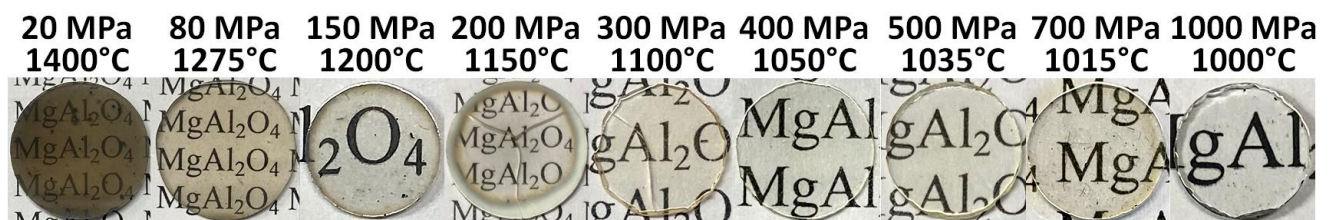
Figure 4.52: Photographs of S25CR-3MS ceramics SPSed for 20 min with different P- T_d conditions
