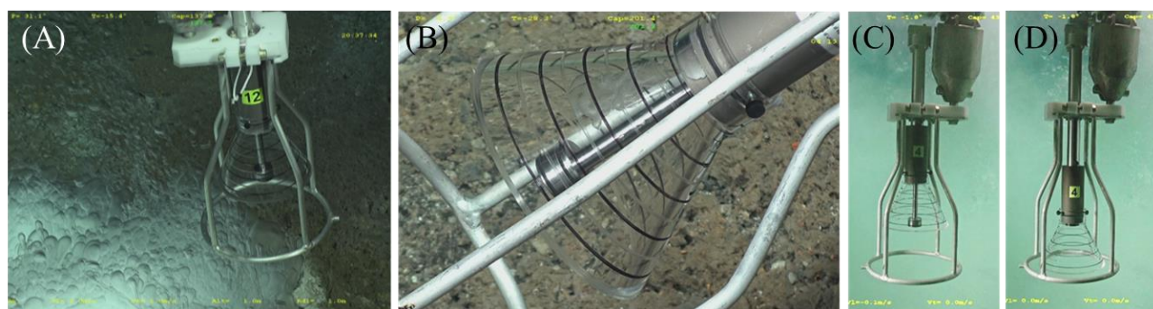
Figure 3. 16. Photography of the PEGAZ sampler taken during an ROV exploration dive. (A) Sampling of liquid \text{CO}_2 droplets above hydrates, (B) sampling of liquid \text{CO}_2 droplets at a direct output from seafloor, (C) PEGAZ sampler in collection position, (D) PEGAZ sampler in activated position.
