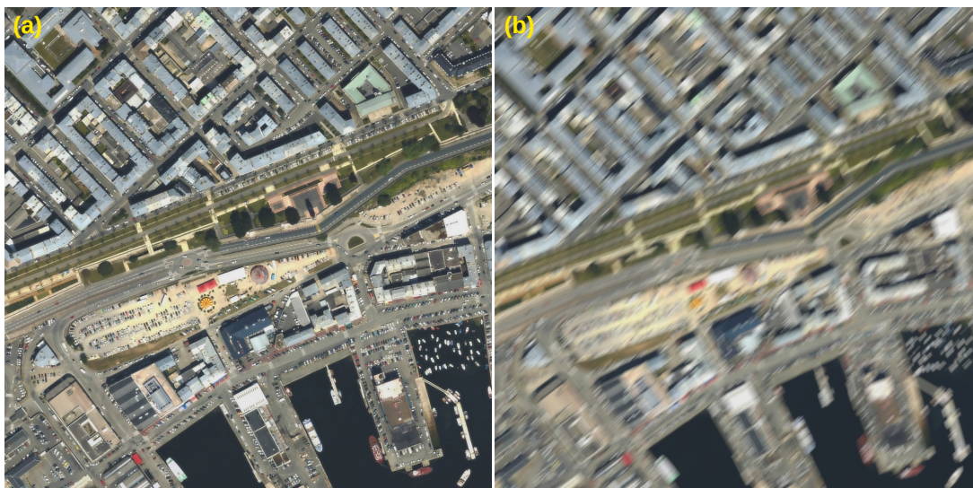
Figure 4.1 – Satellite image of 50-cm resolution of Brest (a) Sharp (b) Motion-blurred
