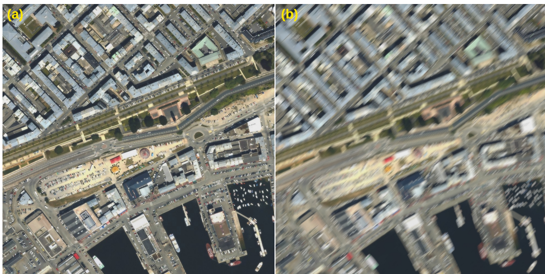
Figure 2 – Satellite image of 50-cm resolution of Brest (a) Sharp (b) Motion-blurred
