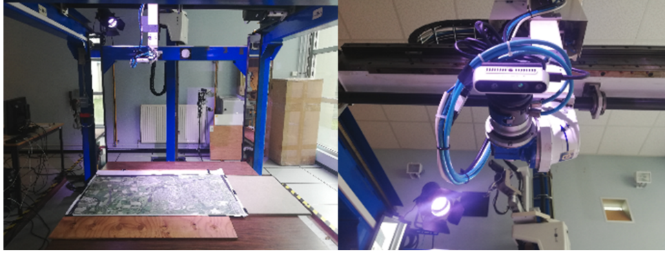
Figure 3.15 – AFMA Cartesian robot positioned above a satellite image, and its INTEL D435 camera mounted on a pan-tilt-roll unit.
