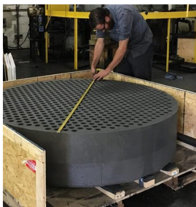
Figure 1.3-8. Heat exchanger made of impregnated graphite from the CGThermal company.[248]
