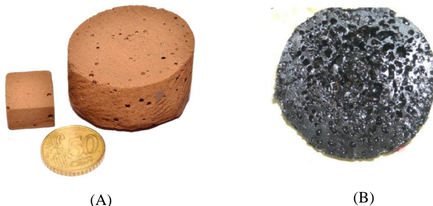
Figure 1.3-6. Example of a PFA-tannin foam (A) [208] and a cross section of a PFA foam for oil recovery (B) [209]
