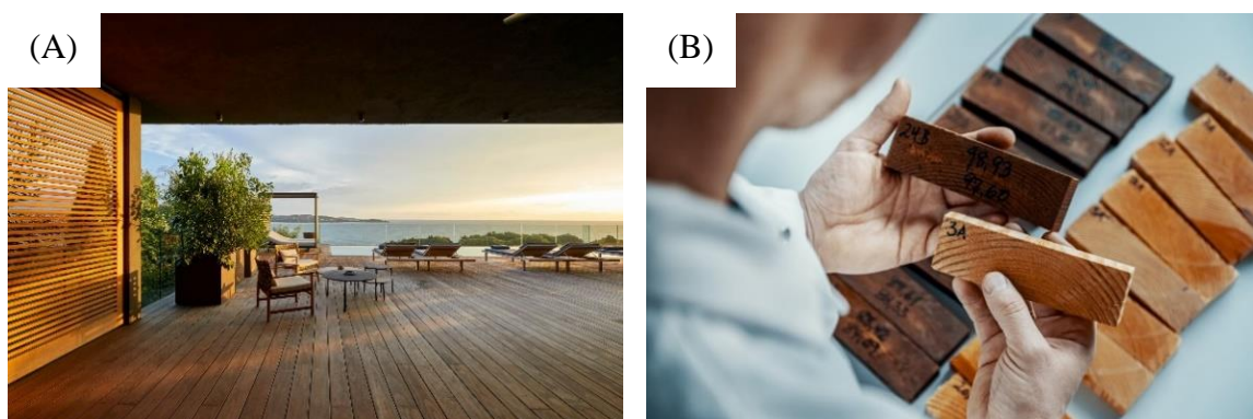
Figure 1.3-3. Pictures of a terrace made of furfurylated wood (Kebony) in Porto-Vecchio (A) [140] and comparison between untreated softwood (light) and a furfurylated one (dark) (B). [141]
