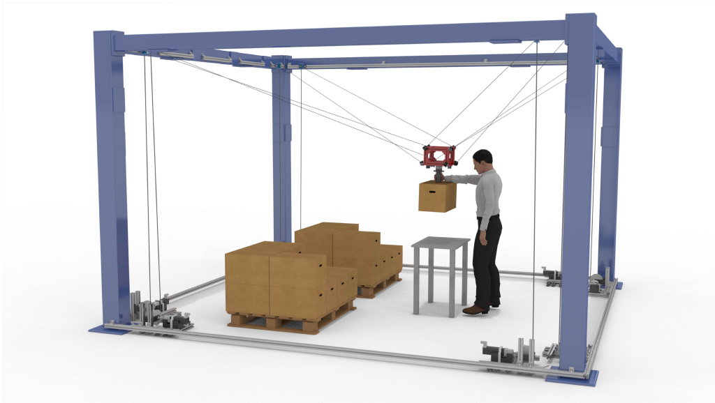
Figure 3.7 – Co-manipulation with a CDPR
