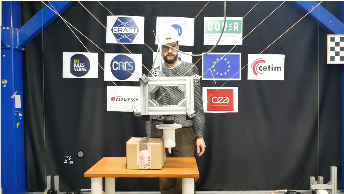
Figure 3.18 – Obstacle interaction while reaching a reference pose
