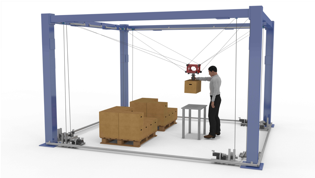
Figure 3.7 – Co-manipulation with a CDPR
